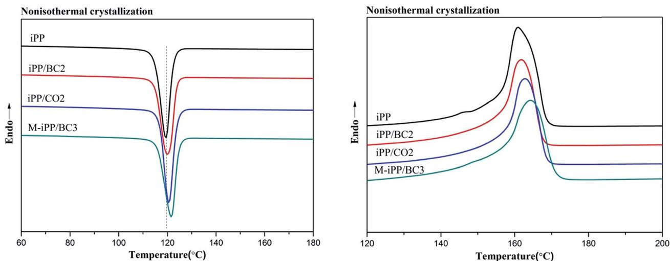
Fig. 3 Non-isothermal crystallization DSC curves of iPP/BC composites (cooling rate 10 °C min<sup>-1</sup>).
