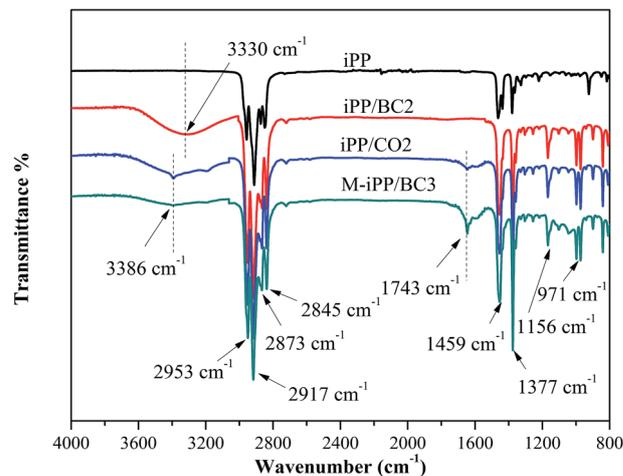
Fig. 1 FT-IR of iPP/BC composites.
