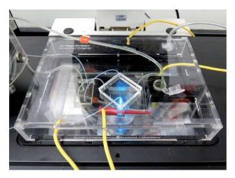
Stage-top incubator with the microfluidic device.
