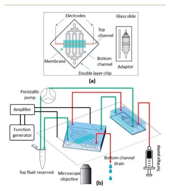
Fig. 1 Schematic of the microfluidic device (a) and the experimental setup (b). Fluid lines for the top and bottom channels are shown in green and red, respectively.
