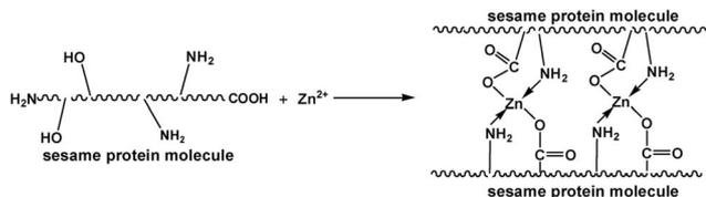
Fig. 5 The reaction process between the sesame protein and zinc oxide.
