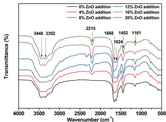
Fig. 4 FTIR spectra of the USP/ZUSP adhesives.
