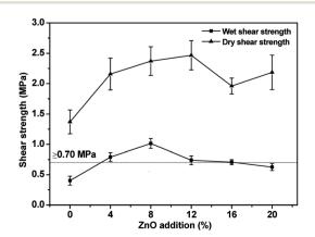
Fig. 3 Bonding strength of the USP/ZUSP adhesives
