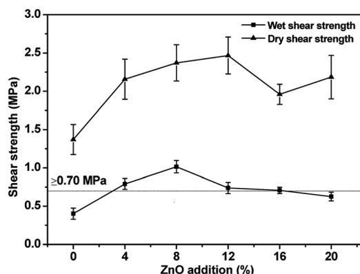
Fig. 3 Bonding strength of the USP/ZUSP adhesives.
