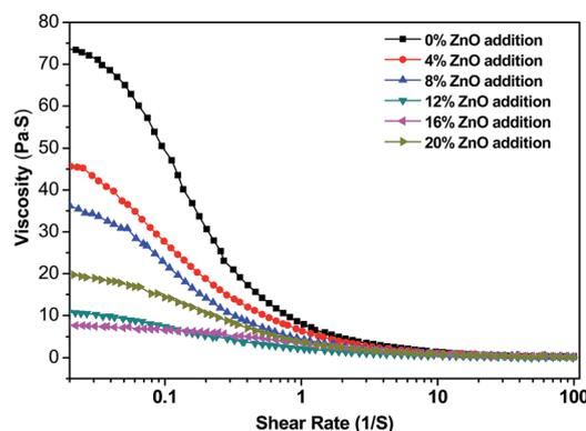
Fig. 2 Apparent viscosity of the USP/ZUSP adhesives.
