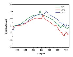
Fig. 4 DSC curve of the Bi-Te-B-Si-P-O glass frit.
