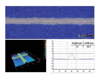
Fig. 9 3D micrographs of the front electrode grid line of SC2.
