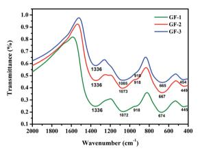
Fig. 3 The infrared spectra of Bi-Te-B-Si-P-O glass frit powders.
