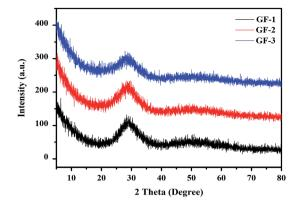
Fig. 2 XRD pattern of different Bi-Te-B-Si-P-O glass frit.
