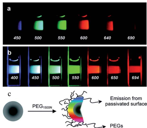
Fig. 1 Aqueous solution of CDs attached to PEG<sub>1500N</sub> (a) excited at 400 nm and photographed through band-pass filters of different wavelengths, as indicated, and (b) excited at the indicated wavelengths and photographed directly. (c) Schematic of passivation of CDs with PEG<sub>1500N</sub>. (Reprinted with permission from ref. 9. Copyright 2006, American Chemical Society.)
