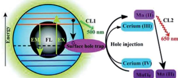
Fig. 3 Schematic illustration of the mechanisms of FL and CL in the CDs— $KMnO_4$  and CDs—cerium(IV) systems. CL1 and CL2 represent two CL pathways in the system. (Reprinted with permission from ref. 61. Copyright 2012, Royal Society of Chemistry.)
