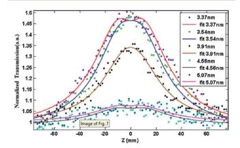
Fig. 11 OA Z-scan of Au–CdSe of different sizes and excitation intensities  $I_0=118~\mu\mathrm{J}.^{101}$
