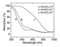
Fig. 5 Optical absorption spectra of Ge nanocrystals embedded in Al<sub>2</sub>O<sub>3</sub> films on quartz substrates (synthesized at room temperature; thickness: 200 nm).72
