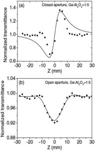
Fig. 6 Z-Scan plots of the Ge nanocrystals embedded in an  $Al_2O_3$  film (Ge:  $Al_2O_3=1:5$ ): (a) closed aperture and (b) open aperture. The solid curves are the theoretical fits.<sup>72</sup>
