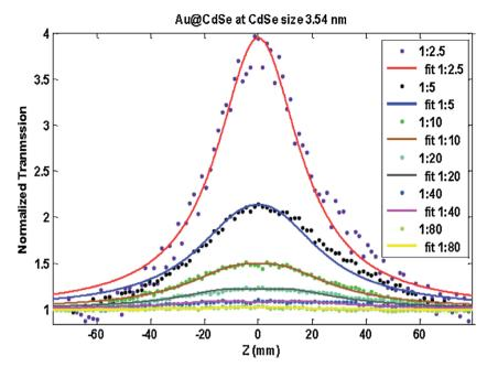
Fig. 12 OA Z-scan transmission of Au-CdSe at 0.31 GW cm<sup>-2</sup> for different concentrations of CdSe (3.54 nm).<sup>101</sup>
