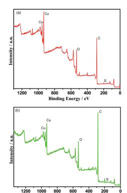
Fig. 7 The elemental binding energy spectra of the RECMs wear surface (a) with the impregnation of SGO and (b) without the impregnation of SGO.
