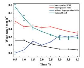
Fig. 4 The carrying-current wear rate over 4 h for the different RECMs.
