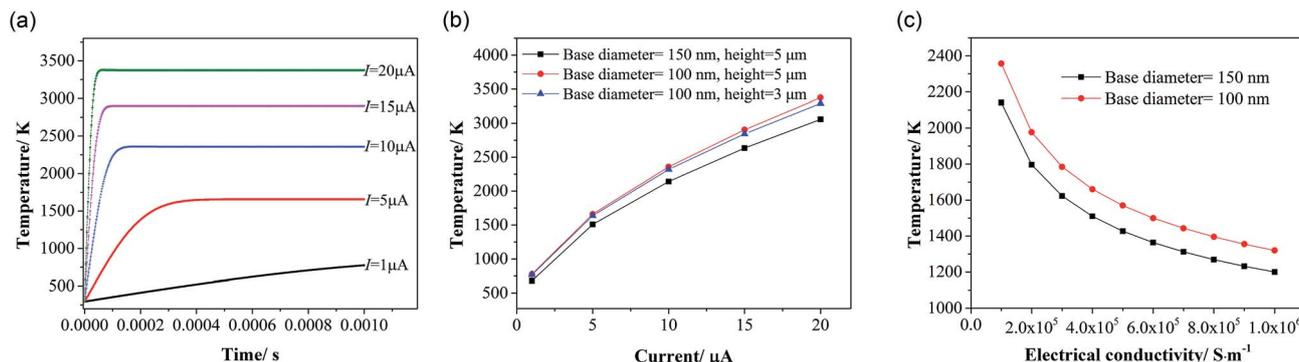
Fig. 8 Finite element analysis results of the effect of Joule heating on maximum temperature of CNF emitters during FE. (a) CNF emitter temperature varies with time at different FE current. (b) Maximum temperature of CNF emitters of different base diameters and height varies with different FE current levels. (c) Temperature varies with electrical conductivity at 10  $\mu\text{A}$  FE current.
