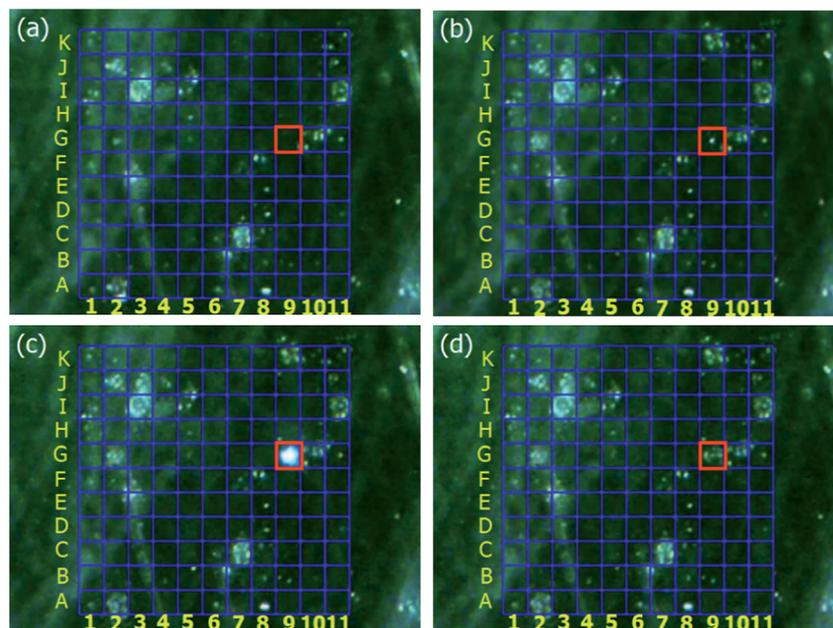
Fig. 3 The entire process of the light emission and the Coulomb explosion at the site G-9: (a) nothing; (b) a light emission occurs; (c) a maximum light emission; (d) an explosion occurs.
