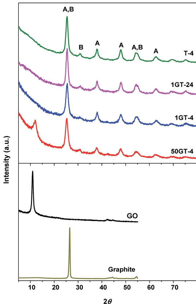
Fig. 4 XRD patterns of GO, starting graphite,  $\text{TiO}_2$  (T-4), and  $\text{GO-TiO}_2$  nanocomposites (1GT-4, 1GT-24 and 50GT-4). A and B indicate the characteristic peaks of anatase and brookite phases, respectively.
