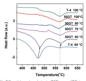
Fig. 11 Differential scanning calorimetry (DSC) curves of TiO $_2$  transitions at 350–650 °C for the samples 50GT (synthesis temperature between 60 and 100 °C) and T-4 (synthesis temperature 60 and 100 °C).
