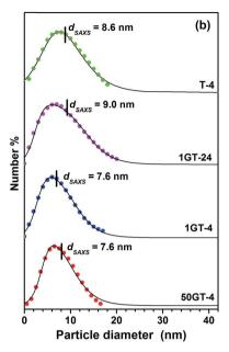
Fig. 3 (a) SAXS curves and (b) correspondent TiO<sub>2</sub> particle size distribution of the GO-TiO<sub>2</sub> composites. The dots indicate the  $D_v(R)$  distribution functions<sup>31,32</sup> and the lines correspond to the log-normal distributions. The average particle diameters,  $d_{SAXS}$ , were calculated from the  $D_v(R)$  distribution functions.
