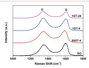
Fig. 6 Raman spectra of GO and GO-TiO2 composites from 100-1800 cm<sup>-1</sup>; D and G band corresponding to sp<sup>3</sup> and sp<sup>2</sup> carbon, respectively.
