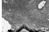
Fig. 1 SEM images of (a) the freeze-dried GO and (b) the nanocomposite prepared with 50 wt% of GO, at 100 °C, for 4 hours (50GT-4).
