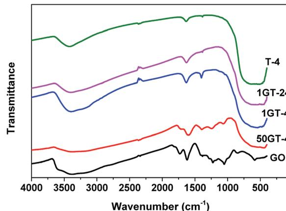
Fig. 5 FTIR transmittance spectra of the starting GO powder (black line), the pure  $\text{TiO}_2$  reference (green line), and of the  $\text{GO-TiO}_2$  nanocomposites 50GT-4 (red line), 1GT-4 (blue line) and 1GT-24 (pink line).
