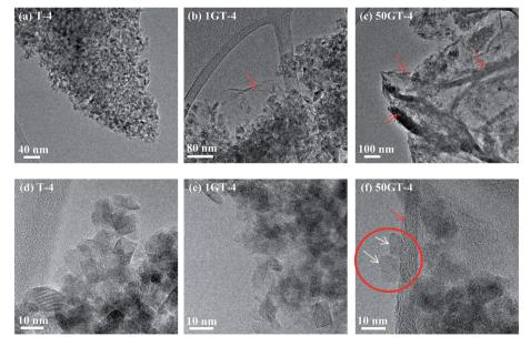
Fig. 2 TEM images of the samples prepared at  $100 \,^{\circ}$ C for 4 hours. (a, d) The pure  $TiO_2$  reference (T-4), (b, e) the nanocomposites with 1 wt% GO (1GT-4), and (c, f) the nanocomposite with 50 wt% GO (50GT-4). Pictures were taken at low (first row) and high magnification (second row). The red arrows point at GO sheets and the white arrows point at  $TiO_2$  crystals.
