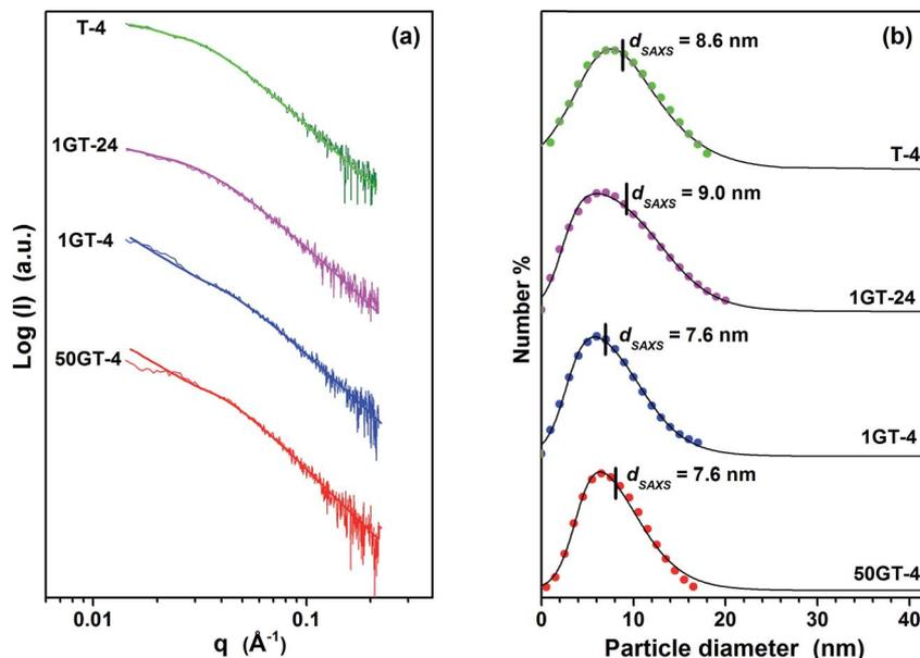
Fig. 3 (a) SAXS curves and (b) correspondent  $\text{TiO}_2$  particle size distribution of the GO- $\text{TiO}_2$  composites. The dots indicate the  $D_v(R)$  distribution functions<sup>31,32</sup> and the lines correspond to the log-normal distributions. The average particle diameters,  $d_{\text{SAXS}}$ , were calculated from the  $D_v(R)$  distribution functions.
