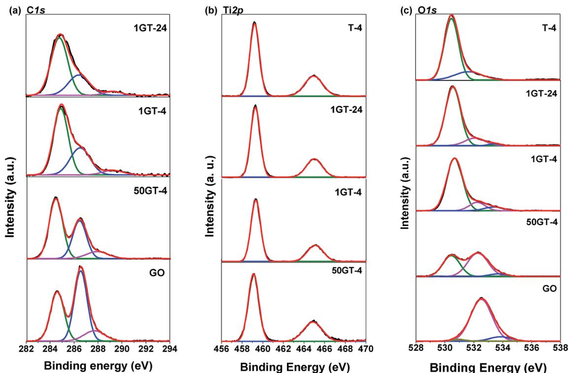
Fig. 7 XPS spectra of GO, T-4, and GO–TiO<sub>2</sub> composites: (a) C1s spectra, (b) Ti2p spectra, and (c) O1s spectra.
