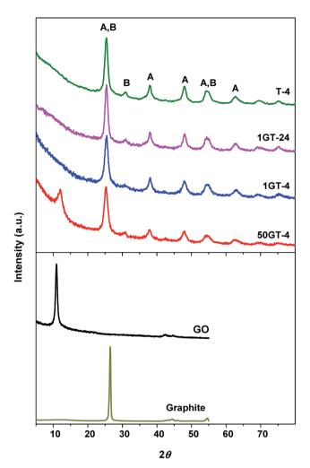
Fig. 4 XRD patterns of GO, starting graphite, TiO<sub>2</sub> (T-4), and GO-TiO<sub>2</sub> nanocomposites (1GT-4, 1GT-24 and 50GT-4). A and B indicate the characteristic peaks of anatase and brookite phases, respectively
