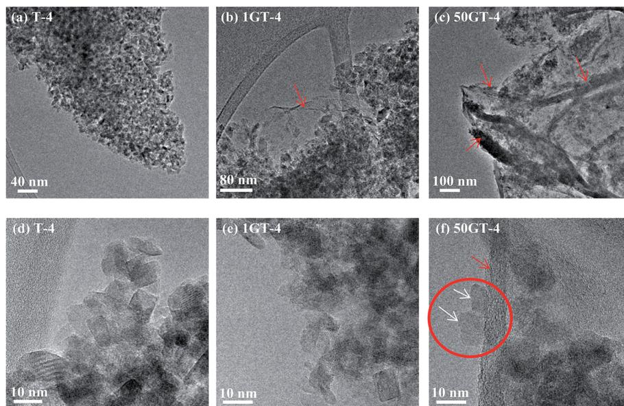
Fig. 2 TEM images of the samples prepared at 100 °C for 4 hours. (a, d) The pure TiO<sub>2</sub> reference (T-4), (b, e) the nanocomposites with 1 wt% GO (1GT-4), and (c, f) the nanocomposite with 50 wt% GO (50GT-4). Pictures were taken at low (first row) and high magnification (second row). The red arrows point at GO sheets and the white arrows point at TiO<sub>2</sub> crystals.
