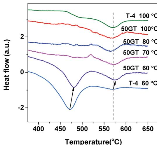
**Fig. 11** Differential scanning calorimetry (DSC) curves of TiO<sub>2</sub> transitions at 350–650 °C for the samples 50GT (synthesis temperature between 60 and 100 °C) and T-4 (synthesis temperature 60 and 100 °C).
