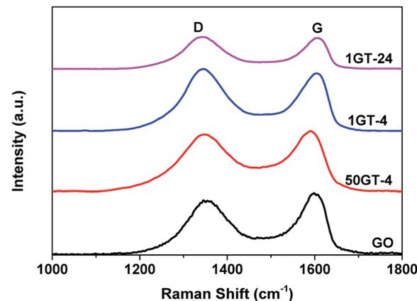
Fig. 6 Raman spectra of GO and  $\text{GO-TiO}_2$  composites from 100–1800  $\text{cm}^{-1}$ ; D and G band corresponding to  $\text{sp}^3$  and  $\text{sp}^2$  carbon, respectively.
