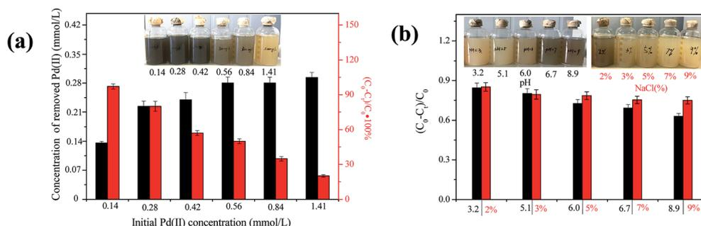
Fig. 6 The effects of initial Pd(II) concentration (a), pH and NaCl concentration (b) on Pd(II) reduction by CNZ-1.
