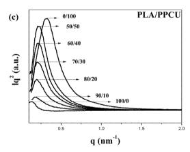
Fig. 9 Crystal X-ray analysis: (a) WAXD patterns of pure PLA and PLA/PPCU blends isothermally crystallized at  $120\,^{\circ}\text{C}$  for 1 h, (b) magnification of the WAXD curve of PLA for the crystalline and amorphous portions, (c) Lorentz-corrected SAXS curves of pure PLA and PLA/PPCU blends.
