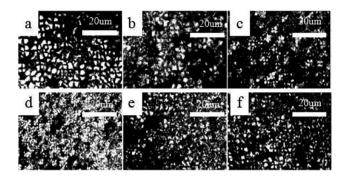
Fig. 10 Spherulitic growth process of pure PLA and PLA/PPCU blends at a crystallization temperature of  $120 \,^{\circ}$ C at 15 min. (a) Pure PLA, (b) 90/10, (c) 80/20, (d) 70/30, (e) 60/40, (f) 50/50.
