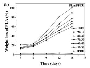
Fig. 12 (a) The weight loss of PLA/PPCU blends and (b) the weight loss of PLA, as a function of time during the enzymatic degradation.
