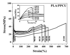
The tensile stress-strain curves of PLA/PPCU
