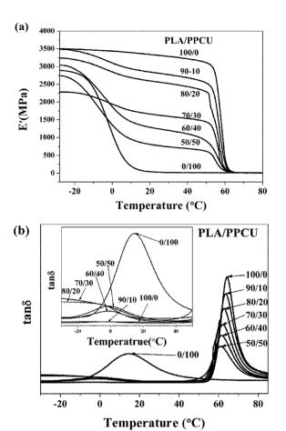
Fig. 11 (a) Dynamic storage modulus, (b)  $\tan\delta$  of pure PLA and PLA/PPCU blends as a function of temperature.
