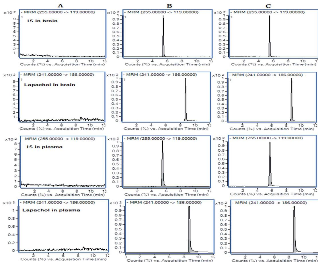
Fig. 2 Representative LC-MS/MS chromatograms for lapachol and IS. (A) Blank samples in rat plasma and dialysate; (B) a spiked dialysate sample with IS and  $50 \text{ ng mL}^{-1}$  of lapachol and a spiked plasma sample with IS and  $1 \text{ } \mu\text{g mL}^{-1}$  of lapachol; (C) random dialysate sample ( $95 \text{ ng mL}^{-1}$ ) at 100 min after administration of lapachol and random plasma sample ( $0.73 \text{ } \mu\text{g mL}^{-1}$ ) at 36 h after administration of lapachol.
