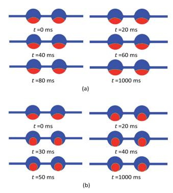
Fig. 8 Phase distribution state via time evolution for the nanofluid flooding case. (a) From random initial state to final intermediate wet state (water contact angle is 90°). (b) From random initial state to final completely water-wet state (water contact angle is 0°).
