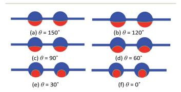
Fig. 9 Final phase distribution at different wettability alteration state (contact angle from  $150^{\circ}$  to  $0^{\circ}$ ).
