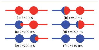
Fig. 6 Flooding process with completely water wet state.
