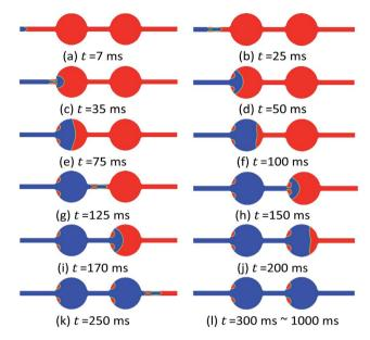
Fig. 5 Flooding process under the intermediate wet state
