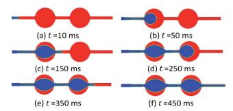
Fig. 4 Flooding process under the completely oil-wet state.
