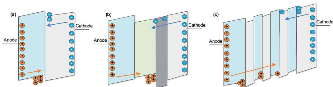
Fig. 3 Schematic diagram of charge distribution in the organic layers before hole and electron combination. (a) Charge distribution in device 1; (b) charge distribution in devices 2 and 3; (c) charge distribution in device 4.
