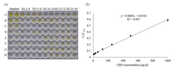
Fig. 5 Standard calibration curve of aptamer-based ELISA method fitted by linear regression using CRP-aptamer-2 as a capture probe. (a) The photo image of the aptamer-based ELISA measurement and (b) the standard calibration curve of the aptamer-based ELISA method. "Standard" indicates the pure CRP protein dilution series coated on the wells, "BS" indicates blind serum samples.
