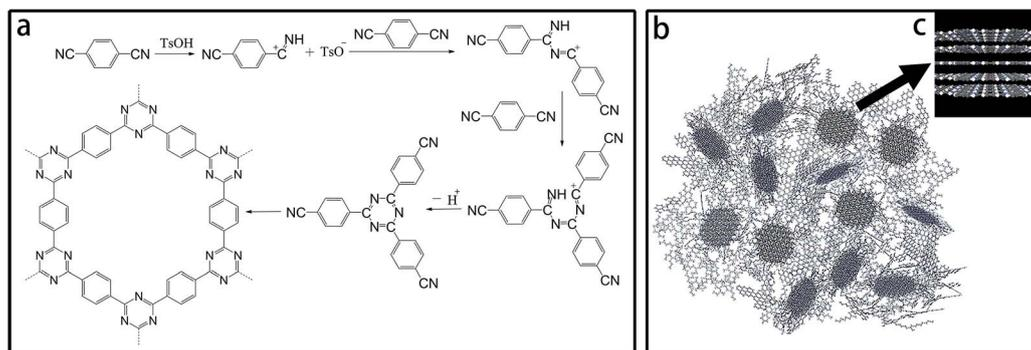
Scheme 1 (a) Trimerization reaction for DCB catalyzed by TsOH; (b) schematic for the CTF structures; and (c) schematic for crystal CTF.
