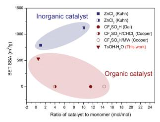
Fig. 1 Comparison of the catalyst to monomer ratio and the BET SSA of various CTF-1s catalyzed by different catalysts (data was derived from the corresponding literature).<sup>23,28–30</sup>
