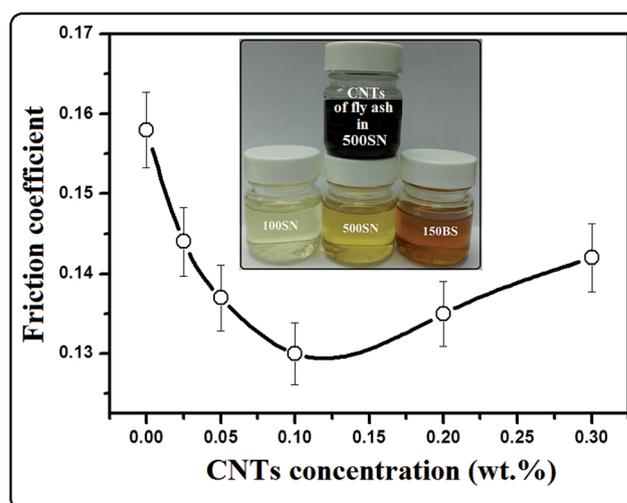
**Fig. 4** Plot of the mean values of the friction coefficient as a function of fly ash-CNTs concentrations in 500SN base oil at a load of 4 N,  $d = 10$  meter,  $R = 2$  mm and linear speed =  $0.5 \text{ cm s}^{-1}$ . The pure and CNTs impregnated 500SN base oils are shown in the inset of this figure. SN100 and 150BS base oils are also shown.
