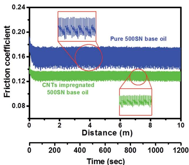
Fig. 5 Plot of the friction coefficient values versus time and distance for pure and CNTs of fly ash impregnated 500SN base oil at a concentration of 0.1 wt%, load = 4 N,  $R = 2$  mm and linear speed =  $0.5 \text{ cm s}^{-1}$ . The plots in the insets are the corresponding extended views for these curves.
