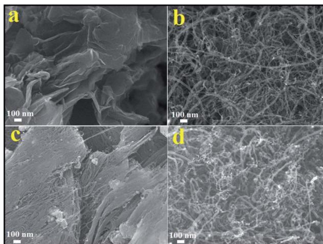
Fig. 1 SEM images at the same magnification of (a) graphene (b) MWCNT, (c) SWCNT and (d) CNTs of oil fly ash.
