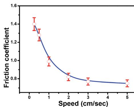
Fig. 7 Plot of the mean values of the friction coefficient as a function of sliding speed for CNTs of fly ash impregnated 500SN base oil obtained at a concentration of 0.1 wt%, load of 4 N,  $d = 10$  meter and  $R = 2$  mm.
