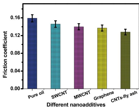
**Fig. 3** Plot of the mean friction coefficient values for different carbon nanomaterial additives impregnated in 500SN base oil at a concentration of 0.1 wt%. The results were obtained at a load of 4 N,  $d = 10$  meter,  $R = 2$  mm and linear speed =  $0.5 \text{ cm s}^{-1}$ .
