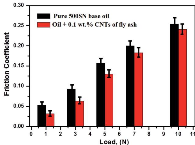
Fig. 6 Plot of the mean values of the friction coefficient as a function of load for pure and CNTs of fly ash impregnated 500SN base oil obtained at a concentration of 0.1 wt%,  $d = 10$  meter,  $R = 2$  mm and linear speed =  $0.5 \text{ cm s}^{-1}$ .
