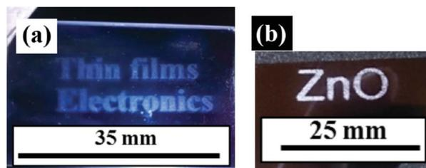
Fig. 7 Printed patterns of PZ4 ink at room temperature and annealed at 200 °C for 3 h. (a) 'Thin films' is printed in 5 passes and 'Electronics' in 10 passes on soda lime glass slide. (b) 'ZnO' pattern is printed in 10 passes on silicon wafer. Both patterns are continuous. The pattern was dried between individual passes using a hot air blower.
