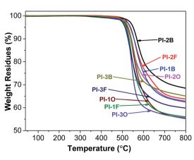
Fig. 4 TGA curves of naphthalene-containing PI films.
