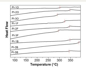
Fig. 5 DSC second heating scan curves of naphthalene-containing PI films with 20 °C min<sup>-1</sup>
