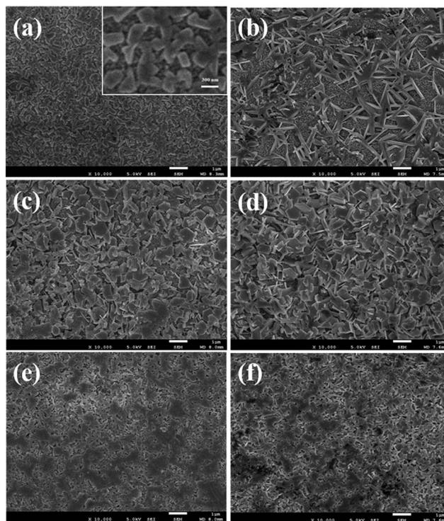
Fig. 1 Top surface SEM images of  $\text{BiI}_3$  (a), one-step solution MBI (b), and two-step MBI prepared with various concentration of MAI:  $3\text{ mg ml}^{-1}$  (c),  $6\text{ mg ml}^{-1}$  (d),  $10\text{ mg ml}^{-1}$  (e), and  $20\text{ mg ml}^{-1}$  (f) on mesoporous  $\text{TiO}_2$  films.
