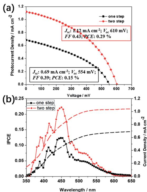
**Fig. 5** (a)  $I$ - $V$  curves for the best performing devices by the one-step and the two-step method, respectively, measured under simulated AM1.5G irradiation. (b) Corresponding IPCEs.
