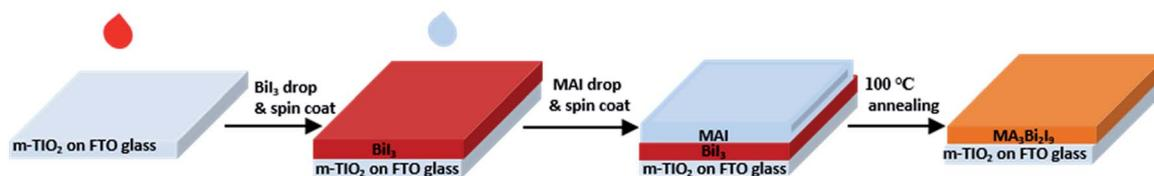
Scheme 1 Fabrication procedure of  $\text{MA}_3\text{Bi}_2\text{I}_9$  on a mesoporous  $\text{TiO}_2$  film through solution deposition and thermal annealing of  $\text{BiI}_3/\text{MAI}$  stacking layer.
