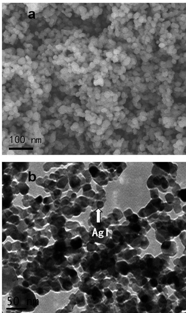
Fig. 1 Images of 0.2-AgI-TiO<sub>2</sub>: (a) SEM, (b) TEM.
