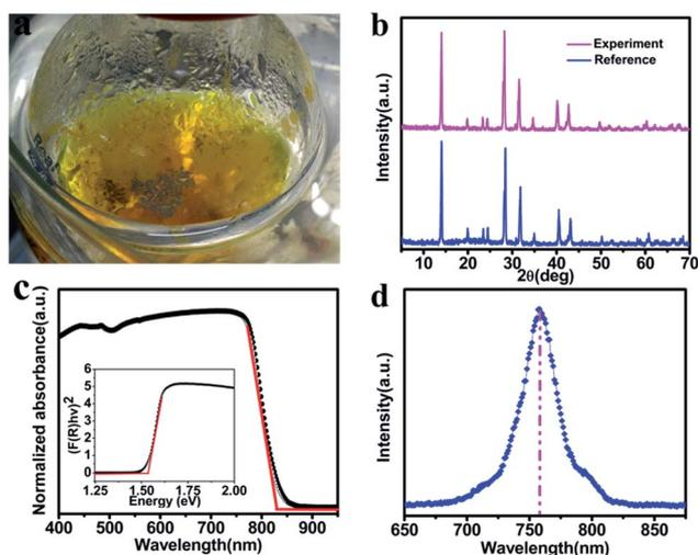
Fig. 7 The photo, X-ray diffraction, UV-vis-NIR absorption spectrum, band gap and PL spectra of MAPbI<sub>3</sub> wafer.
