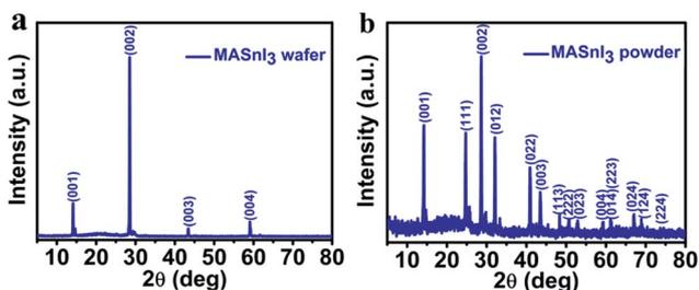
Fig. 2 X-ray diffraction of (a) the  $\text{MASnI}_3$  wafer and (b)  $\text{MASnI}_3$  powder grounded from a wafer.
