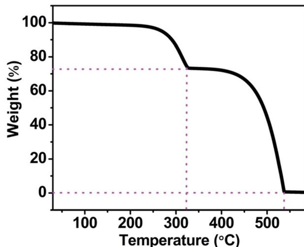
Fig. 6 Thermal gravimetric (TGA) data for MASnI<sub>3</sub> wafer.
