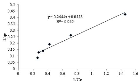
Fig. 9 Langmuir isotherm for adsorption of MB by TMAN.
