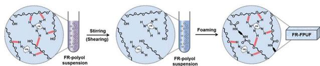
Scheme 2 The illustration of shear-responsive internal network in FR-polyol suspensions and FR-FPUFs.
