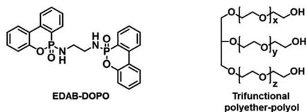
Scheme 1 Chemical structures of EDAB-DOPO and polyether-polyol.
