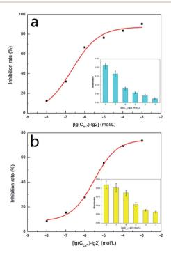
Fig. 5 The detection of screened out metal ions. (a) The effect of different concentrations of Ag $^+$  on GOx activity, a series of concentrations of Ag $^+$  ranging from 2  $\times$  10 $^{-8}$  to 2  $\times$  10 $^{-3}$  mol L $^{-1}$ . (b) The effect of different concentrations of Cu $^{2+}$  on GOx activity, a series of concentrations of Cu $^{2+}$  ranging from 2  $\times$  10 $^{-8}$  to 2  $\times$  10 $^{-3}$  mol L $^{-1}$ .
