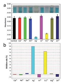
Fig. 4 The screening of GOx metal ion inhibitors. (a) UV-vis absorption spectra (652 nm) and the related optical images of control group (GOx untreated by metal ions) and experimental groups (GOx treated by metal ions). (b) Effects of metal ions (2 mM) on GOx activity. The metal ions are Ca<sup>2+</sup>, Pb<sup>2+</sup>, Mn<sup>2+</sup>, Ag<sup>+</sup>, Al<sup>3+</sup>, Cu<sup>2+</sup>, Mg<sup>2+</sup> and Zn<sup>2+</sup>.
