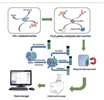
Fig. 1 Schematic illustration of the proposed method for the metal ion inhibitors screening of glucose oxidase.
