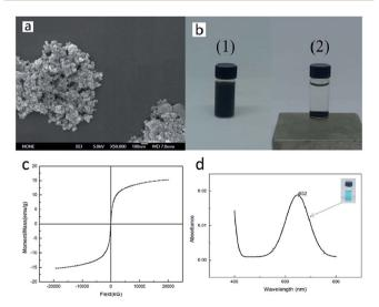
Fig. 2 (a) SEM image of the synthesized Fe<sub>3</sub>O<sub>4</sub> particles. (b) Response of Fe<sub>3</sub>O<sub>4</sub> MNPs to a magnet (NdFeB). (1) Fe<sub>3</sub>O<sub>4</sub> MNPs dispersion liquid. (2) Status that Fe<sub>3</sub>O<sub>4</sub> MNPs had been gravitated by the magnet. (c) The magnetization curve for Fe<sub>3</sub>O<sub>4</sub> MNPs. (d) UV-vis absorption spectra (400-800 nm) and the related optical images of the nano-Fe<sub>3</sub>O<sub>4</sub> catalyzed color reaction.
