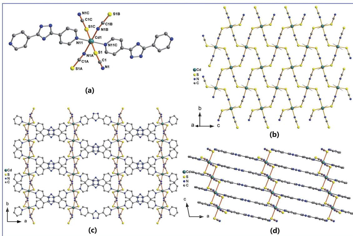
Fig. 2 (a) View of the coordination environment of cadmium cations in **2**, symmetry codes:  $A\ x, -y + 2, z + 1/2$ ,  $B\ -x + 1/2, y - 1/2, -z - 1/2$ ,  $C\ -x + 1/2, -y + 3/2, -z$ ; (b) 2-D (4, 4) layer consisting of  $\mu_2$ -SCN<sup>-</sup> anions and Cd(II) cations, the wedge-like lines represent the 4,4'-Hbpt ligands; (c) view of the 3D network of **2** along the *c*-axis; (d) view of the 3D network of **2** along the *b*-axis. All H atoms are omitted for clarity.
