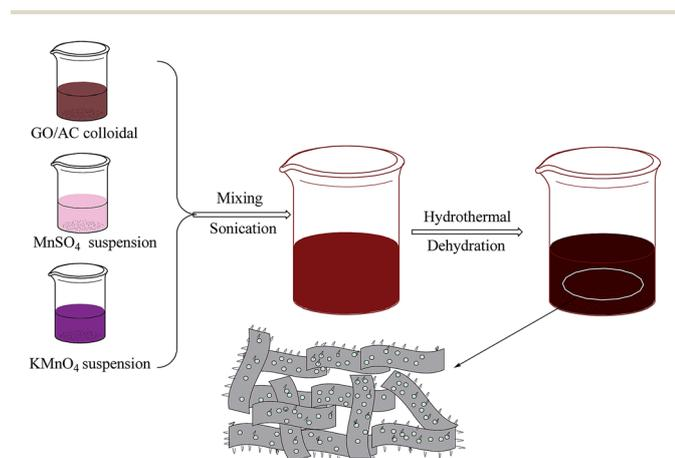
Fig. 1 Illustration of the fabrication process of GR/AC/MnO<sub>2</sub> composites.
