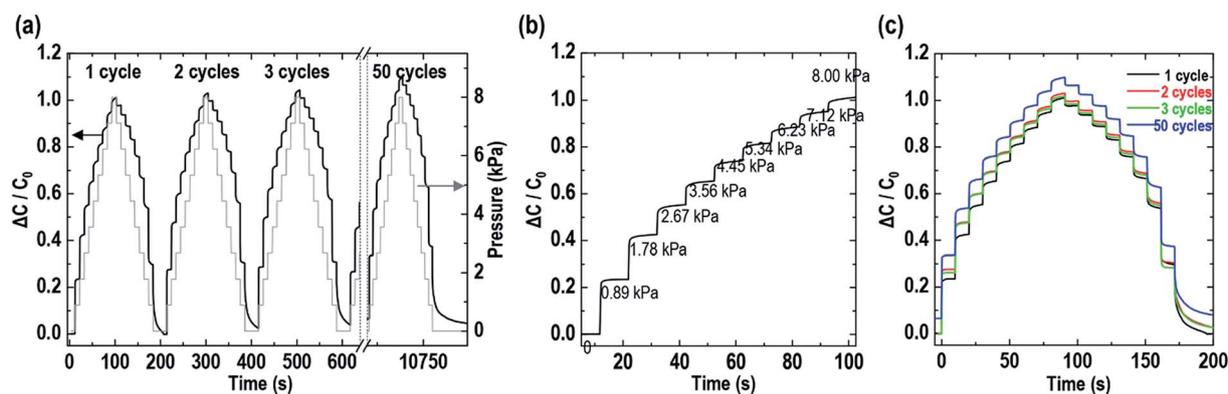
Fig. 4 (a) Step-by-step repeatability test as measured by  $\Delta C/C_0$  over repeated loading/unloading cycles. (b) Force step used in the step-by-step repeatability test. (c) Overlapping graphs of the step-by-step repeatability test.
