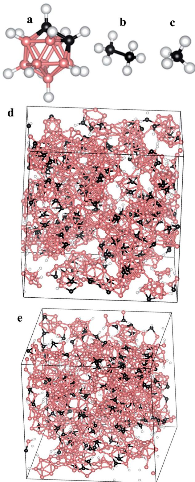
Fig. 2 Molecular structure of the initial molecules. (a)  $B_{10}C_2H_{12}$ ; (b)  $CH_3CH_3$ ; (c)  $CH_4$ ; (d) structure of a sample model (d1.7–H23.5–B/C4.8) produced by LAMMPS; (e) structure of the same sample model (d1.7–H23.5–B/C4.8) after VASP relaxation. In all cases: boron: pink, carbon: black, hydrogen: white.
