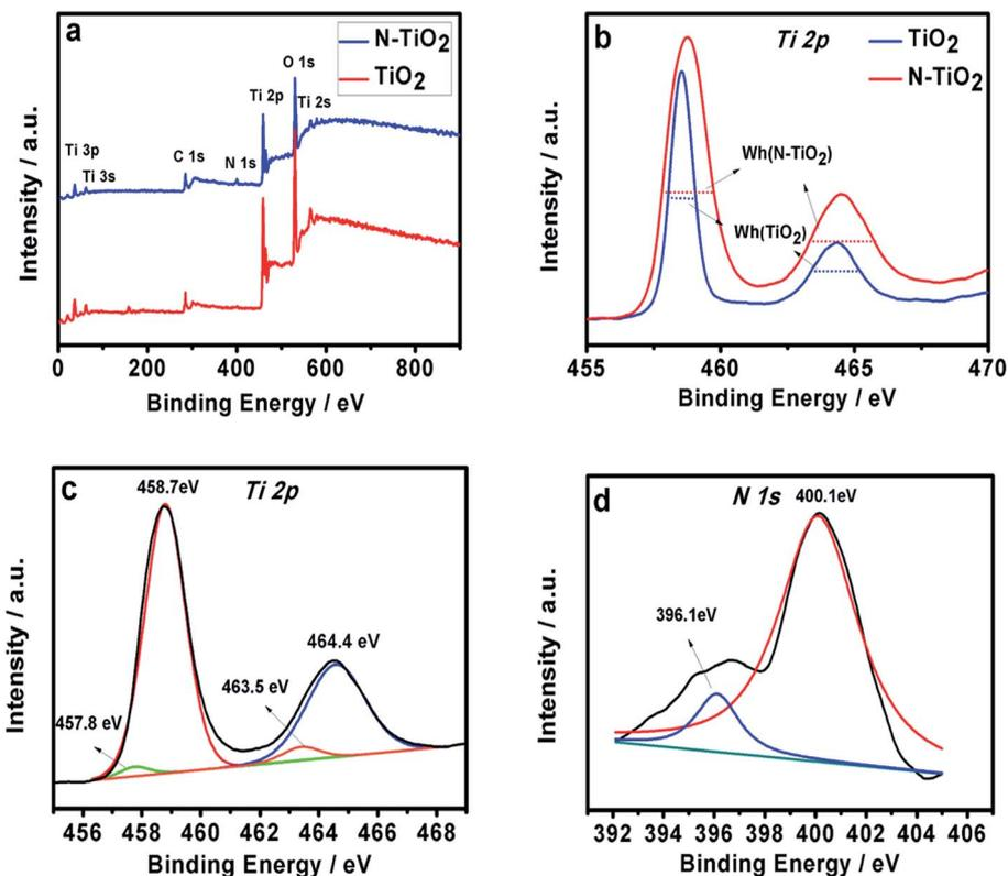
Fig. 3 (a) XPS survey spectra of  $\text{TiO}_2$  and N-doped  $\text{TiO}_2$ . High-resolution XPS spectra of Ti 2p peaks of  $\text{TiO}_2$  (b) and N-doped  $\text{TiO}_2$  as well as Ti 2p (c) and N 1s (d) peaks of N- $\text{TiO}_2$ .
