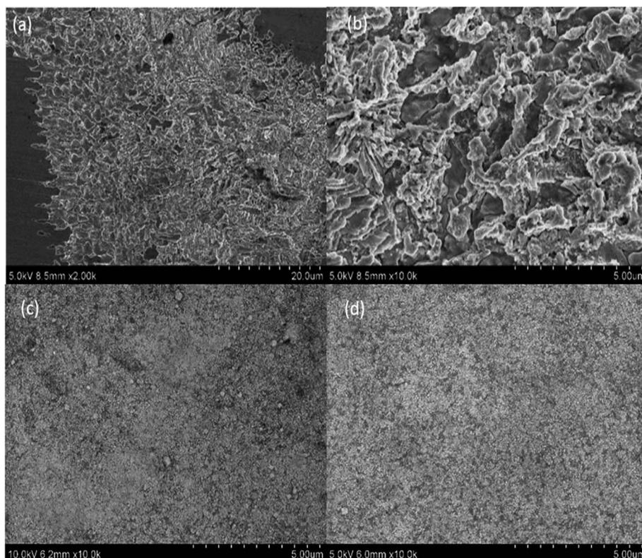
Fig. 8 SEM surface images of (a, b) CAW, (c) TiO<sub>2</sub>-coated CAW and (d) N-TiO<sub>2</sub>-coated CAW after potentiodynamic polarization tests.
