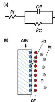
Fig. 7 (a) Equivalent circuit used for fitting the experimental data of TiO<sub>2</sub> and N-TiO<sub>2</sub> coatings, (b) corresponding equivalent circuit principle diagram.
