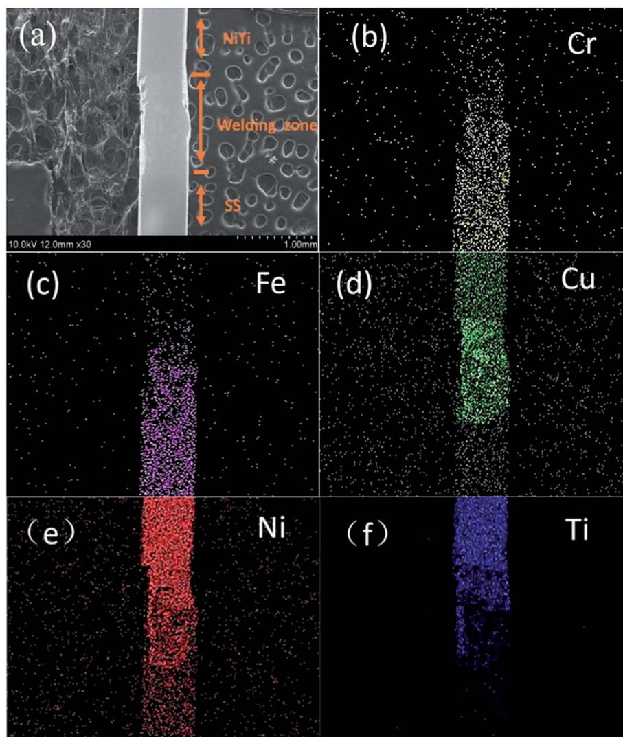
Fig. 1 SEM image (a) and the corresponding EDS mapping images of laser-welded composite arch wire (b–f).
