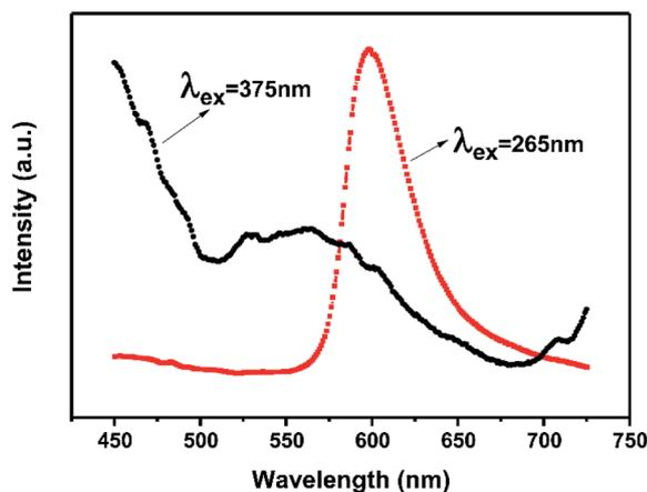
Fig. 3 Emission spectra of  $\text{Ca-}\alpha\text{-sialon}:\text{0.02Mn}^{2+}$  phosphors under excitation of 375 nm and 265 nm.
