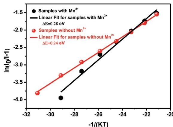
Fig. 6 Activation energy  $\Delta E$  of thermal quenching of Ca- $\alpha$ -sialon:0.08Eu<sup>2+</sup> with ( $x = 0.02$ ) and without Mn<sup>2+</sup> phosphors.
