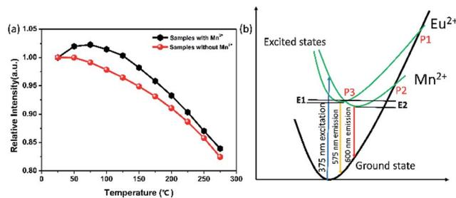
Fig. 4 (a) Temperature dependent luminescence of  $\text{Ca-}\alpha\text{-sialon}:\text{0.08Eu}^{2+}$  with ( $x = 0.02$ ) and without  $\text{Mn}^{2+}$  phosphors measured under 375 nm excitation. (b) Schematic illustration of the configuration coordinate diagram of energy transfer in the  $\text{Ca-}\alpha\text{-sialon}:\text{0.08Eu}^{2+},\text{0.02Mn}^{2+}$  phosphor.
