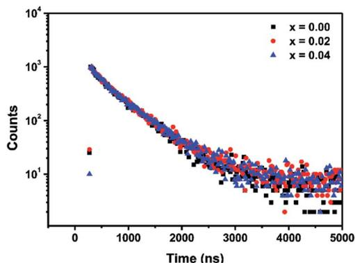
Fig. 7 Decay curves of three phosphor samples: Ca- $\alpha$ -sialon:0.08Eu<sup>2+</sup> (black dots), Ca- $\alpha$ -sialon:0.08Eu<sup>2+</sup>,0.02Mn<sup>2+</sup> (red dots) and Ca- $\alpha$ -sialon:0.08Eu<sup>2+</sup>,0.04Mn<sup>2+</sup> (blue dots), detected at  $\lambda_{em} = 570$  nm and  $\lambda_{ex} = 375$  nm.
