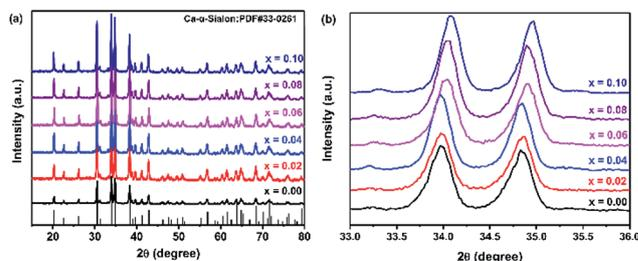
Fig. 1 (a) XRD patterns of  $\text{Ca-}\alpha\text{-sialon}:\text{0.08Eu}^{2+},x\text{Mn}^{2+}$  phosphors with various  $\text{Mn}^{2+}$  concentrations ( $x = 0.00\text{--}0.10$ ); (b) magnified regions of the XRD patterns in the  $2\theta$  range of 33–36°.
