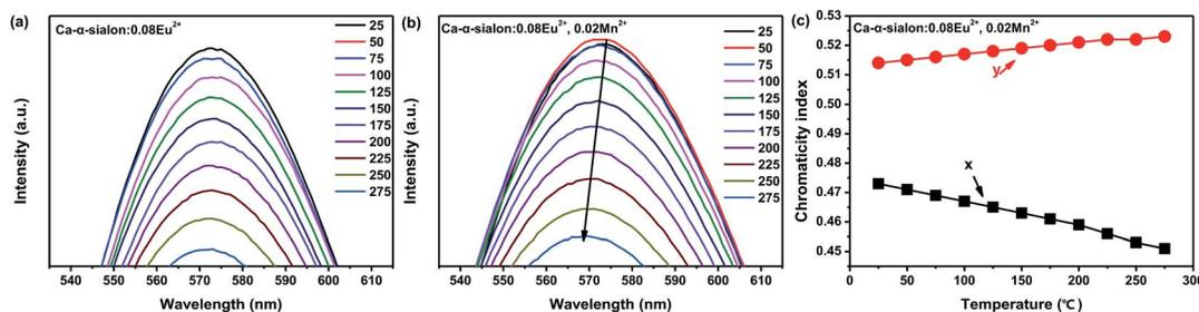
Fig. 5 (a) and (b) PL emission spectra of Ca- $\alpha$ -sialon:0.08Eu<sup>2+</sup> without and with Mn<sup>2+</sup> phosphors ( $x = 0.02$ ) as a function of temperature. (c) CIE chromaticity coordinates of Ca- $\alpha$ -sialon:0.08Eu<sup>2+</sup>, 0.02Mn<sup>2+</sup> phosphor versus temperature.
