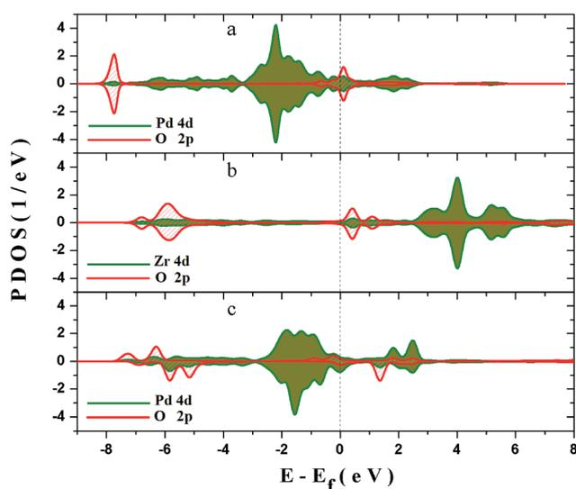
Fig. 7 PDOS for different adsorption configurations: (a)  $\text{O}_2$  adsorbed on cus-Pd site of PdO (101) surface; (b)  $\text{O}_2$  adsorbed on cus-Zr site of  $\text{Pd}_{5/6}\text{Zr}_{1/6}\text{O}$  (101) B surface and (c)  $\text{O}_2$  adsorbed on cus-Pd site of  $\text{Pd}_{5/6}\text{Zr}_{1/6}\text{O}$  (101) B surface.
