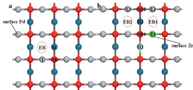
Fig. 5 Top view of the adsorption sites of (a) PdO (001) surface and (b) Pd<sub>8/9</sub>Zr<sub>1/9</sub>O (001) surface.
