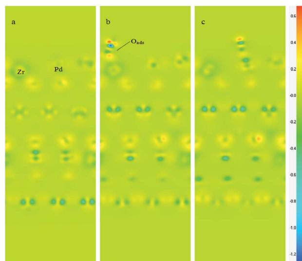
Fig. 8 The section patterns for difference electron density of (a)  $\text{Pd}_{5/6}\text{Zr}_{1/6}\text{O}$  (101) B surface; (b)  $\text{Pd}_{5/6}\text{Zr}_{1/6}\text{O}$  (101) B surface with adsorbed  $\text{O}_2$  on cus-Zr and (c)  $\text{Pd}_{5/6}\text{Zr}_{1/6}\text{O}$  (101) B surface with adsorbed  $\text{O}_2$  on cus-Pd.
