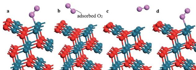
Fig. 3 The configuration of the PdO after adsorbing a O<sub>2</sub> on the (a) 4f O; (b) 4f Pd; (c) cus O and (d) cus Pd site, respectively.
