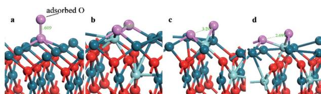
**Fig. 6** The configuration of the PdO after adsorbing a O<sub>2</sub> on the (a) H site of PdO (001) surface; (b) H1 and (c) H2 site of Pd<sub>8/9</sub>Zr<sub>1/9</sub>O (001) surface and (d) H site of Pd<sub>7/9</sub>Zr<sub>2/9</sub>O (001).**Table 5** Calculated formation energies (in kJ mol<sup>-1</sup>) of PdO and Zr-doped-PdO surfaces
