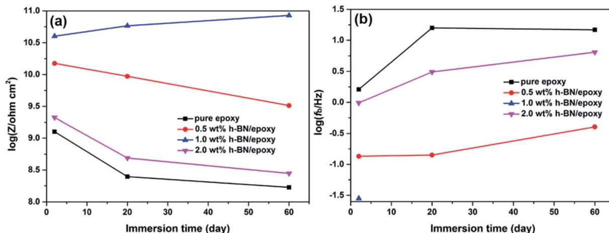
Fig. 9 Variations of (a)  $\log Z$  at 0.01 Hz and (b)  $\log f_b$  as a function of immersion time for pure epoxy, 0.5 wt% h-BN/epoxy, 1.0 wt% h-BN/epoxy and 2.0 wt% h-BN/epoxy coatings in 3.5 wt% NaCl solution.
