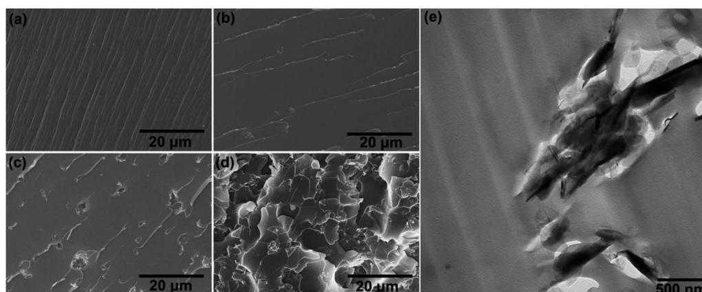
Fig. 6 The SEM images of fracture surface for different samples, (a) pure epoxy, (b) 0.5 wt% h-BN/epoxy, (c) 1.0 wt% h-BN/epoxy, (d) 2.0 wt% h-BN/epoxy coatings and (e) TEM image of 0.5 wt% h-BN/epoxy coating.
