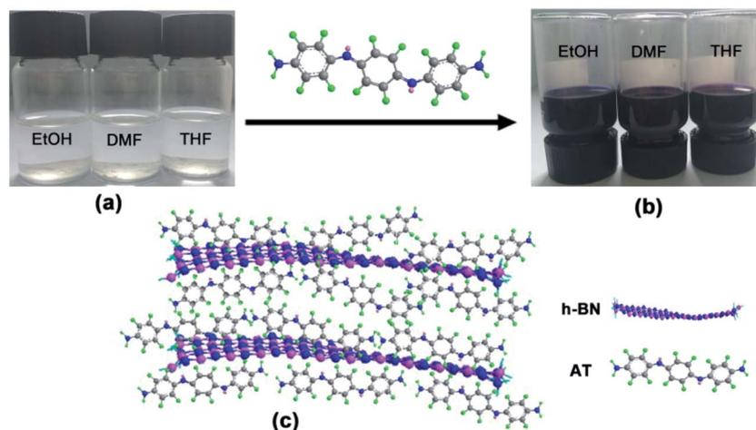
Fig. 1 The dispersion of h-BN nanoplatelets in different solvents without (a) or with (b) AT as dispersant and corresponding schematic illustration of  $\pi$ - $\pi$  interactions between h-BN and AT (c).
