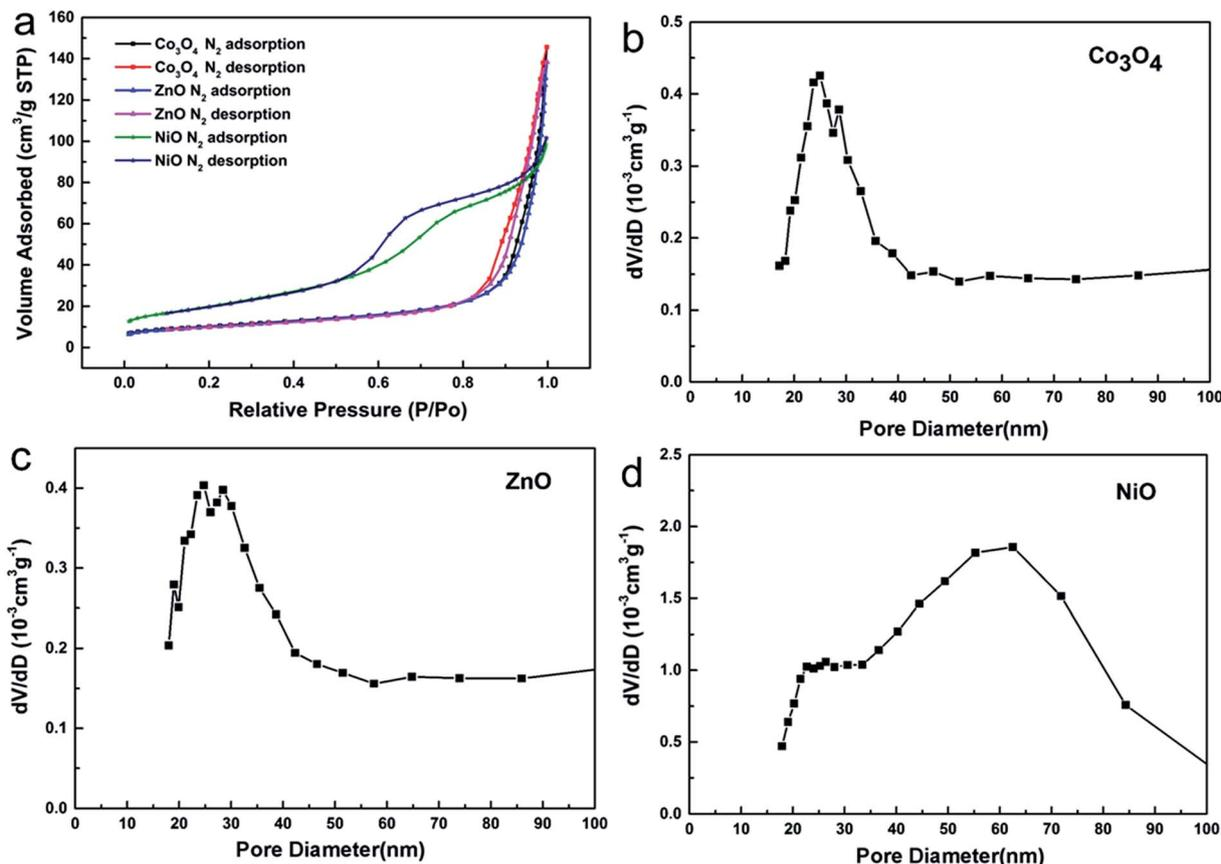
Fig. 4 (a)  $\text{N}_2$  adsorption–desorption isotherms of the  $\text{Co}_3\text{O}_4$  nanowires,  $\text{ZnO}$  nanosheets and  $\text{NiO}$  nanosheets. (b–d) The BJH pore size distribution curves of  $\text{Co}_3\text{O}_4$ ,  $\text{ZnO}$  and  $\text{NiO}$ .
