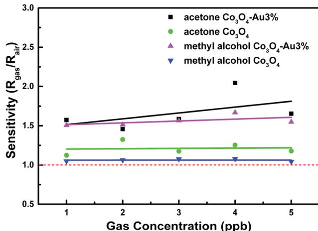
Fig. 9 The sensing responses to 1–5 ppb acetone and methyl alcohol at each optimum operating temperature of Co<sub>3</sub>O<sub>4</sub> and Co<sub>3</sub>O<sub>4</sub>-Au.
