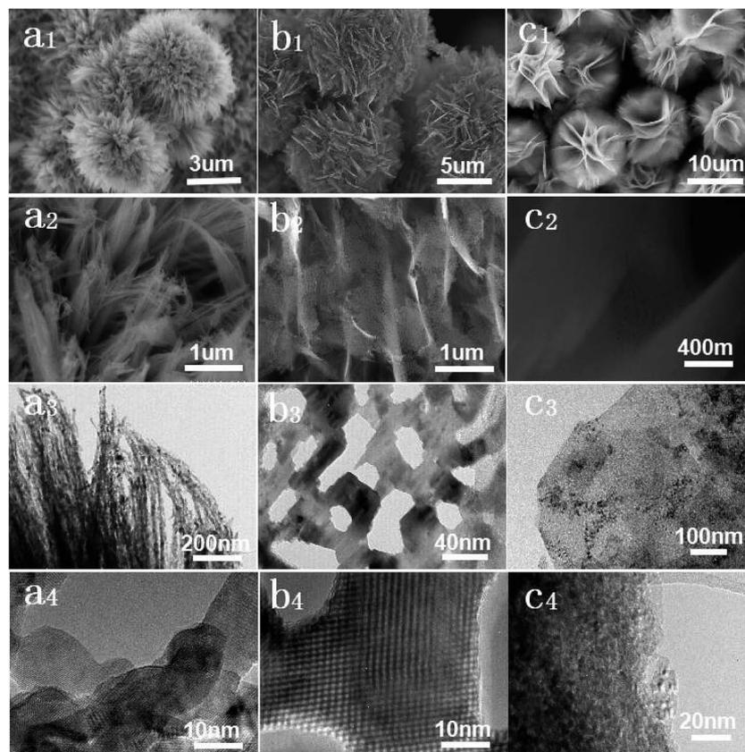
Fig. 2 SEM, TEM and HRTEM images of the as-synthesized (a<sub>1</sub>–a<sub>4</sub>)  $\text{Co}_3\text{O}_4$  flower-like structures with porous nanowires, (b<sub>1</sub>–b<sub>4</sub>) ZnO porous nanosheets, and (c<sub>1</sub>–c<sub>4</sub>) NiO porous nanosheets. The images above clearly show the porous and hierarchical characteristics of the prepared samples.
