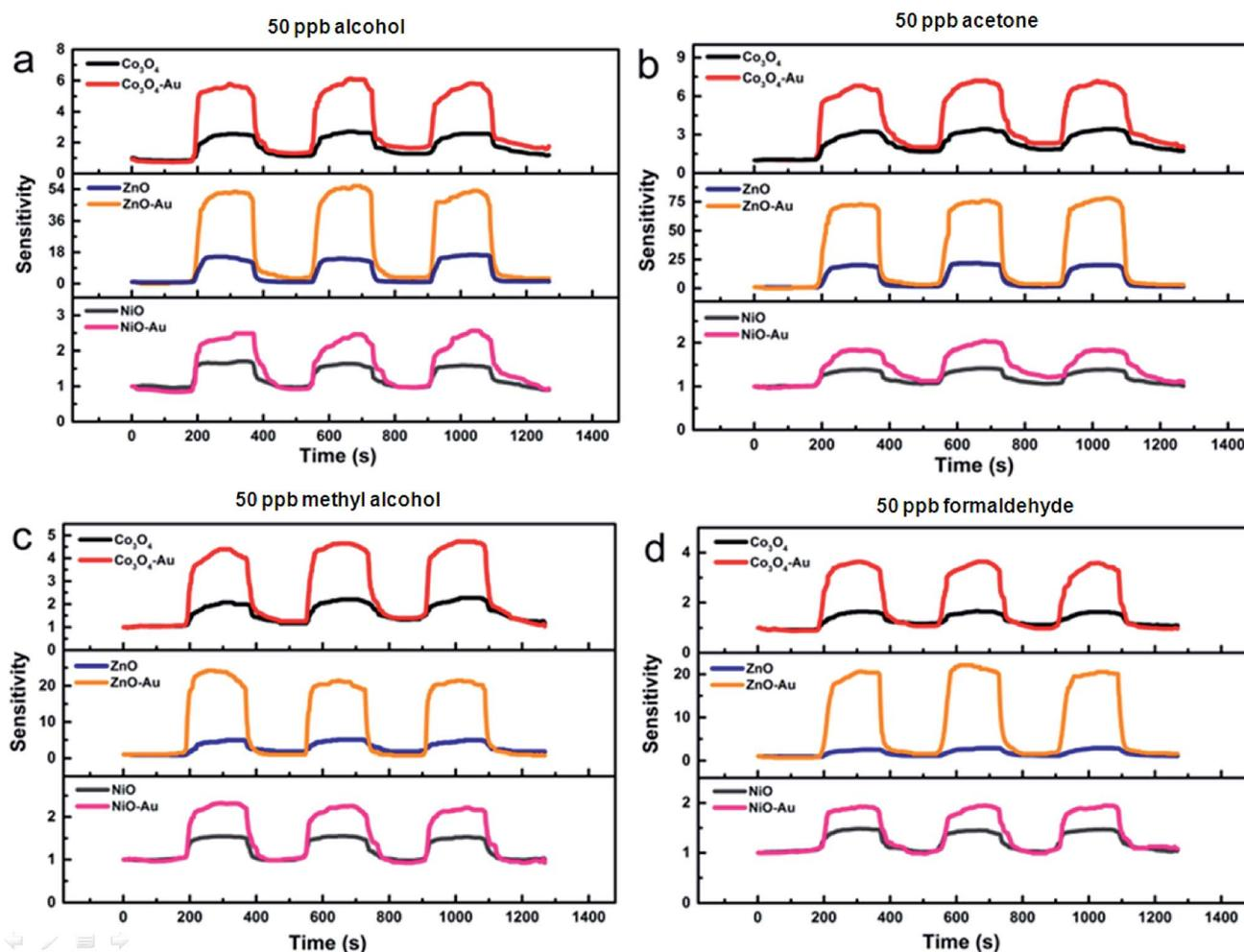
Fig. 8 The sensing responses of  $\text{Co}_3\text{O}_4/\text{Co}_3\text{O}_4\text{-Au}$ , ZnO/ZnO–Au and NiO/NiO–Au to 50 ppb (a) alcohol, (b) acetone, (c) methyl alcohol, and (d) formaldehyde at each optimum operating temperature.
