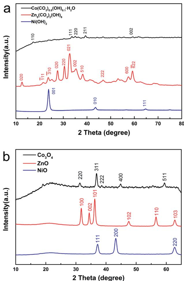
Fig. 1 (a) XRD patterns of the precursors  $\text{Co}(\text{CO}_3)_{0.5}(\text{OH})_{0.1} \cdot \text{H}_2\text{O}$ ,  $\text{Zn}_5(\text{CO}_3)_2(\text{OH})_6$  and  $\text{Ni}(\text{OH})_2$ . (b) XRD patterns of as-synthesized  $\text{Co}_3\text{O}_4$ ,  $\text{ZnO}$  and  $\text{NiO}$ , achieved by annealing the precursors.
