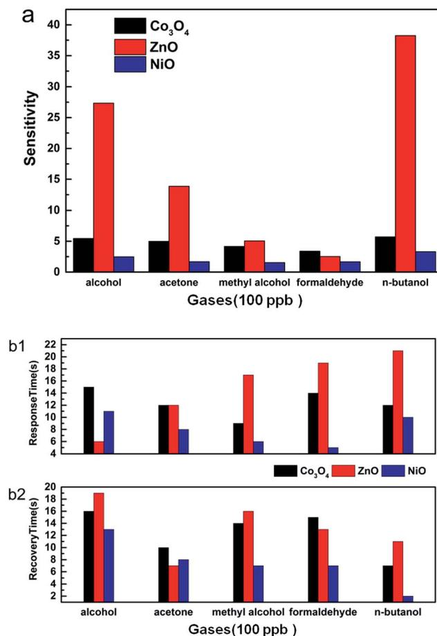
Fig. 6 (a) Gas sensitivities and (b<sub>1</sub> and b<sub>2</sub>) response and recovery times of porous  $Co_3O_4$ , porous ZnO, and porous NiO.
