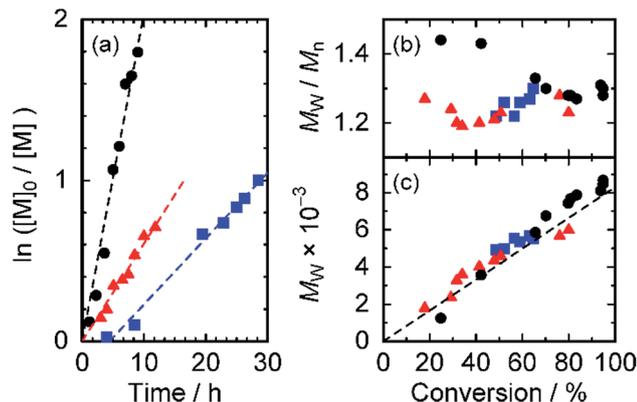
Fig. 2 (a) First-order kinetic plot of  $\ln([M]_0/[M])$  versus time, (b) evolution of polydispersity index, and (c) number-average molecular weight for the RAFT polymerization of DDA. The broken line in (c) represents the theoretical prediction. Reaction conditions: (black circles)  $[DDA]/[CTA-Me]/[AIBN] = 204/4.7/1$  in toluene, (red triangles)  $[DDA]/[CTA-Me]/[AIBN] = 210/4.8/1$  in DMF, and (blue squares)  $[DDA]/[CTA-Pr]/[AIBN] = 210/4.8/1$  in DMF.
