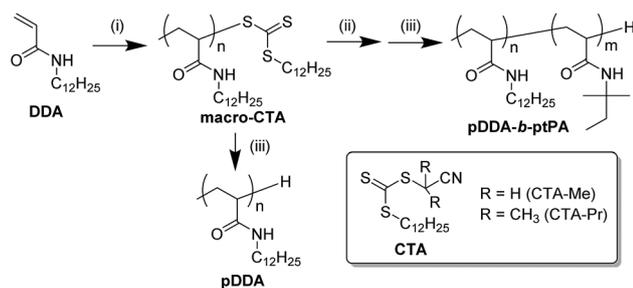
**Scheme 1** Synthesis route of macro-CTA and block copolymers pDDA-*b*-ptPA: (i) AIBN, CTA, toluene or DMF, 60 °C, 24–48 h; (ii) tPA, AIBN, toluene, 60 °C, 20 h; (iii) tris(trimethylsilyl)silane, AIBN, toluene, 60 °C, 4 h.
