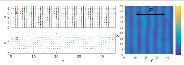
Fig. 5 EC with a positive dielectric LC is shown here. The projected nematic directors (black bars) are shown in panel a, and the corresponding flows (blue arrows) are shown in panel b. The reflection of polarized incident light (polarization shown as a black arrow) is plotted in panel c. It is noted that the EC rolls shown in panel c are moving in the +y direction, which is a typical character of the TW mode, and the net directional flow seen in panel b is in the -y direction.
