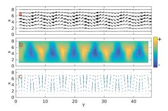
Fig. 2 The typical EC with negative dielectric LCs is shown here. Panel a is the x-y projection of the directors, while panel c is the x-y projection of the flows. The middle panel b shows the bound charges seen in the x-y plane, for which they are calculated according to eqn (5).
