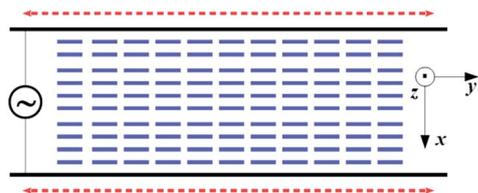
Fig. 1 The equilibrium configuration of EC with a negative dielectric LC. The red dashed arrows indicate the planar wall anchoring in the  $y$  direction, and the blue bars are the negative dielectric LCs. An AC electric field is applied along the  $x$  direction,  $\vec{E}_x$ .
