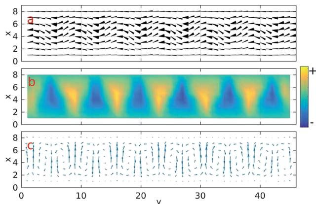
Fig. 2 The typical EC with negative dielectric LCs is shown here. Panel a is the  $x$ - $y$  projection of the directors, while panel c is the  $x$ - $y$  projection of the flows. The middle panel b shows the bound charges seen in the  $x$ - $y$  plane, for which they are calculated according to eqn (5).
