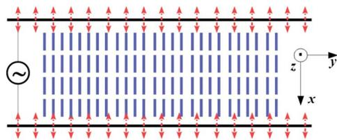
Fig. 4 The equilibrium configuration of EC with a positive dielectric LC. The red dashed arrows indicate the homeotropic wall anchoring in the  $x$  direction, and the blue bars are the positive dielectric LCs. An AC electric field is applied along the  $x$  direction  $\vec{E}_x$ .
