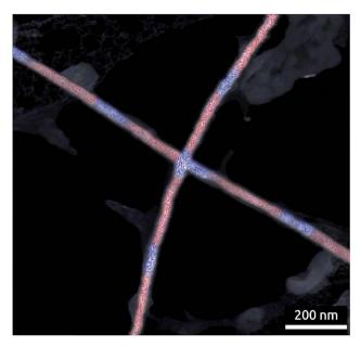
Fig. 10 HAADF-STEM image superimposed with elemental maps showing the local distribution of Co (red) and Cu (blue) in  $Ni_{60}Co_{40}/Cu$  nanowires of 40 nm diameter. Individual EDX maps of the elements Ni, Co and Cu are presented in Fig. S5.†
