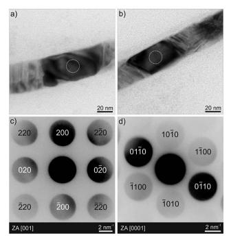
Fig. 9 Representative TEM results of  $Ni_{60}Co_{40}/Cu$  nanowire of 40 nm diameter. The bright-field TEM images in (a and b) show crystallites in different sections of one nanowire. The corresponding (contrast inverted) CBED patterns in (c and d) are obtained from the nanowire segments with darker contrast in (a and b), and correspond to the [001] zone axis of fcc Cu (ICSD 43493) and to the [0001] zone axis of hcp NiCo (ICSD 102567), respectively.
