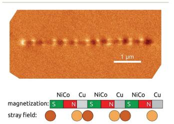
Fig. 11 Top, magnetic force micrograph of an isolated  $Ni_{60}Co_{40}/Cu$  wire of 40 nm diameter (shown in Fig. 8). Lower panel, schematic representation of how the pattern observed in MFM originates from the alternation of magnetized and non-magnetic segments.
