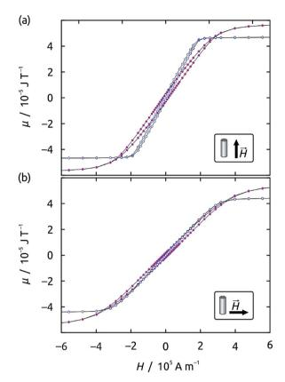
Fig. 4 Magnetic hysteresis curves obtained for  $Ni_{60}Co_{40}$  (empty blue circles) and  $Ni_{42}Co_{58}$  (full purple disks) wires of 300 nm diameter by SQUID magnetometry with the external field applied either parallel to the wires' long axis (a) or perpendicular to it (b).
