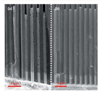
Fig. 1 Co nanowires of 300 nm diameter grown inside the porous template at an applied potential of -1.0 V (a) and -1.1 V (b) vs. Ag/AgCl. The latter value results in smoother, more uniform wires. A thin sputtered Au film and short Au segment subsequently grown (galvanically) as the electrical contact are observable near the lower extremity of the pores.
