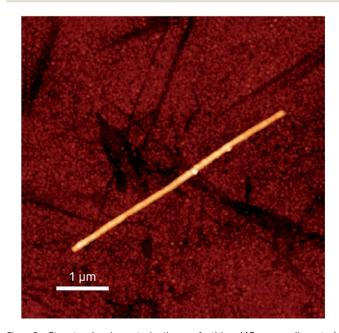
8 Structural characterization of thin (40 nm diameter), segmented NiCo/Cu wires isolated from the matrix. Atomic force micrograph of a straight segment, investigated by magnetic force microscopy in Fig. 11.
