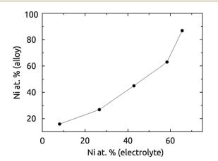
Fig. 3 Composition of the NiCo wires (diameter 300 nm) deposited, determined by atomic absorption spectroscopy (AAS), as a function of the electrolyte composition.
