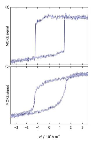
Fig. 6 Magnetic hysteresis loops recorded by magneto-optical magnetometry (MOKE) on individual wires of 300 nm diameter and composition (a)  $\rm Ni_{60}Co_{40}$  and (b)  $\rm Ni_{82}Co_{18}$ . The switching is perfectly abrupt with the softest composition (a) and more gradual for less optimal materials (b). The vertical axis is in arbitrary units: in MOKE magnetometry, a signal proportional to the local magnetization is recorded as a polarized light intensity.
