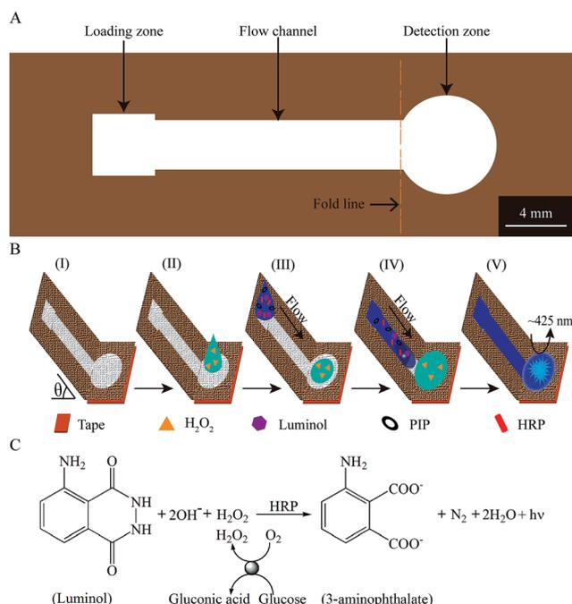
**Fig. 1** Schematic of the cloth-based device design and sensing principle. (A) The layout for the cloth-based device before folding. It includes a loading zone, flow channel and detection zone. (B) The  $\text{H}_2\text{O}_2$  sensing principle using the cloth-based device. (C) The possible reaction mechanism for the  $\text{H}_2\text{O}_2$  or glucose sensing.
