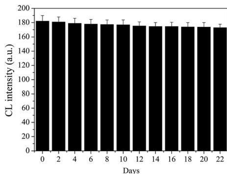
Fig. 6 Storage stability of the cloth-based devices for the determination of  $\text{H}_2\text{O}_2$  (pH of test/substrate solutions-7.5/8.0, [luminol]-1.0 mM, [HRP]-0.3 g  $\text{L}^{-1}$ , [PIP]-0.2 mM, [ $\text{H}_2\text{O}_2$ ]-0.5 mM, angle of inclination- $50^\circ$ , volumes of test/substrate solutions-30  $\mu\text{L}$ /35  $\mu\text{L}$ ). The error bar represents the standard deviation of five independent measurements.
