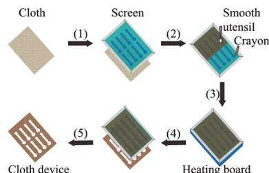
**Fig. 2** Schematic of the wax screen-printing for fabrication of the unfolded cloth-based devices. (1 and 2) The screen is placed on the cloth, and rubbed with a crayon and smooth utensil in turn. (3) The cloth is placed onto the heating board together with the screen. (4 and 5) The cloth and screen are removed from the heating board, and then separated from each other.
