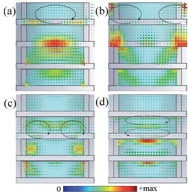
Fig. 9 Vector distributions of the electric field, magnetic field, induced currents and power loss density at resonance frequencies: (a) 10.0 GHz, (b) 14.5 GHz, (c) 21.1 GHz and (d) 27.2 GHz. (a) and (b) are  $y$ - $z$  cutting planes along with the electric field orientation, (c) and (d) are  $x$ - $z$  cutting planes along with the magnetic field orientation.
