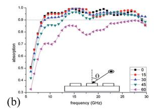
Fig. 8 Absorption spectra of the ILMMA at different (a) polarization angles ( $\varphi$ ) of 0–90° and (b) incident angles ( $\theta$ ) of 0–60°.
