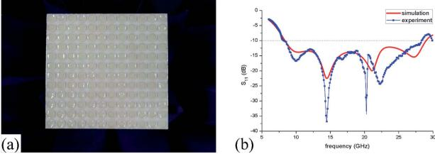
Fig. 12 (a) Photograph of the ILMMA prototype (b) simulated and measured reflection coefficient (S<sub>11</sub>).
