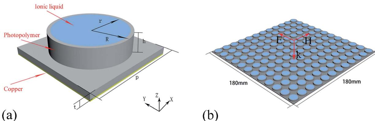
Fig. 4 (a) Schematic of an ILMMA unit cell and (b) the periodic array.
