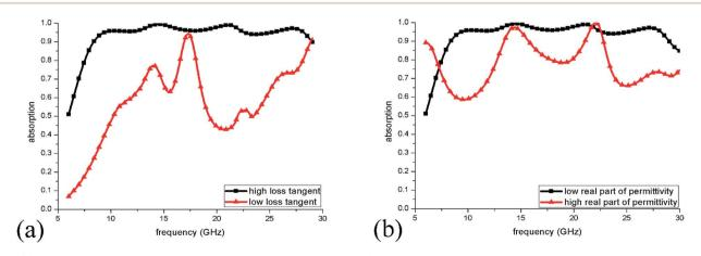
Fig. 11 (a) Absorption spectra of ILMMA with decreased loss tangent of IL. (b) Absorption spectra of ILMMA with increased real part of permittivity of IL.
