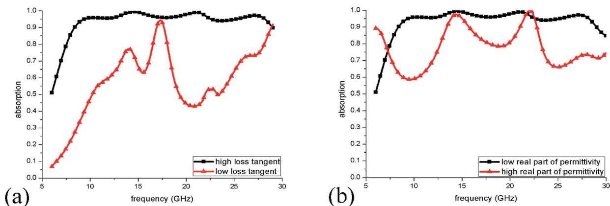
Fig. 11 (a) Absorption spectra of ILMMA with decreased loss tangent of IL. (b) Absorption spectra of ILMMA with increased real part of permittivity of IL.
