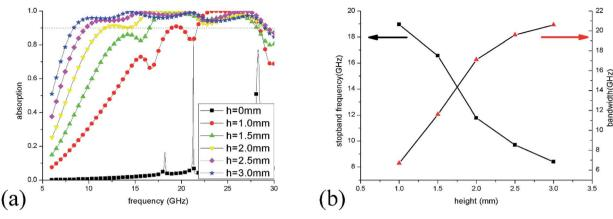
Fig. 5 Changes of microwave absorption by height of IL cylinders. (a) Changes of absorption spectra when changing height of IL cylinders by 6 steps (0, 1.0, 1.5, 2.0, 2.5 and 3.0 mm) and fixing radius as 5.5 mm. (b) Changes of stopband frequency and absorption bandwidth with cylinder height increases.
