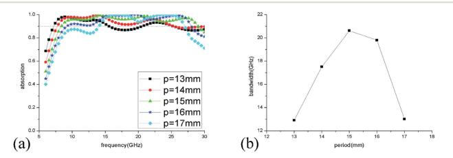
Fig. 7 Changes of microwave absorption by unit period. (a) Absorption spectra of ILMMA at different unit periods (13, 14, 15, 16, and 17 mm) when cylinder height is 3 mm and radius is 5.5 mm. (b) Changes of the absorption bandwidth with the period increases.
