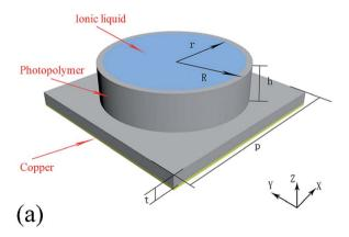
(a) Schematic of an ILMMA unit cell and (b) the periodic array.
