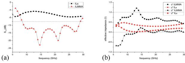
Fig. 10 (a) Reflection spectra of IL layer of 4 mm on copper surface and the corresponding ILMMA in frequency range of 6–30 GHz. (b) Calculated effective impedances of IL layer and ILMMA.
