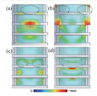
Fig. 9 Vector distributions of the electric field, magnetic field, induced currents and power loss density at resonance frequencies: (a)  $10.0 \, \text{GHz}$ , (b)  $14.5 \, \text{GHz}$ , (c)  $21.1 \, \text{GHz}$  and (d)  $27.2 \, \text{GHz}$ . (a) and (b) are y-z cutting planes along with the electric field orientation, (c) and (d) are x-z cutting planes along with the magnetic field orientation.
