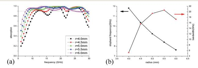
Fig. 6 Changes of microwave absorption by diameter of IL cylinders. (a) Changes of absorption spectra when changing radius of IL cylinders by 5 steps (4.0, 4.5, 5.0, 5.5 and 6.0 mm) and fixing height as 3 mm. (b) Changes of stopband frequency and absorption bandwidth with cylinder radius increases.
