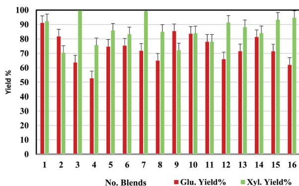
Fig. 1 Glucose and xylose yields from acidolysis of sixteen MSW blends after pretreatment with selected conditions ( $[\text{C}_2\text{C}_1\text{Im}]\text{Cl}$ , 160 °C, 2 h) at 10 mL scale (see Table 1 for sample IDs and compositions).
