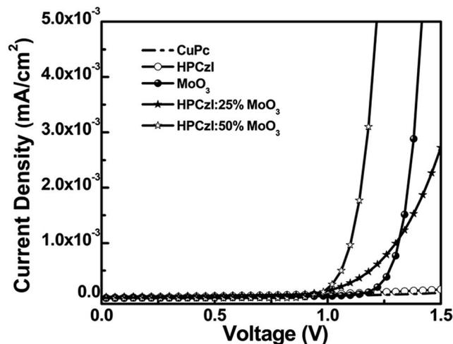
Fig. 5 The *J*–*V* characteristics of hole-only devices with structure of ITO/NPB (10 nm)/X (60 nm)/NPB (100 nm)/Al (100 nm). The X are pure films of CuPc, HPCzI, MoO<sub>3</sub> and MoO<sub>3</sub> doped HPCzI films.
