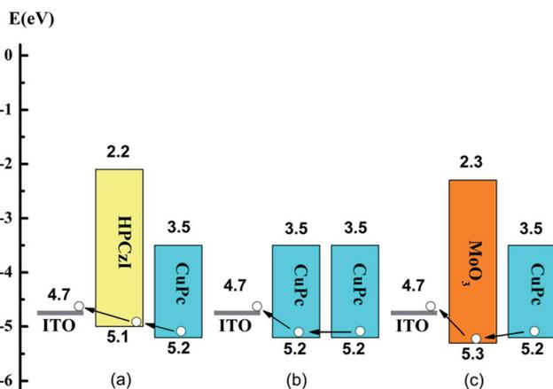
Fig. 4 Hole collection in devices with different ABL: (a) HPCzI, (b) CuPc, (c) MoO<sub>3</sub>.
