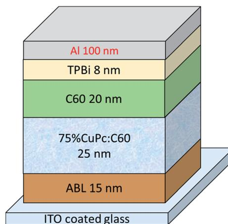
Fig. 1 Device structure of organic solar cells, with CuPc, HPCzI, MoO<sub>3</sub> and MoO<sub>3</sub> doped HPCzI as anode buffer layer (ABL), respectively.
