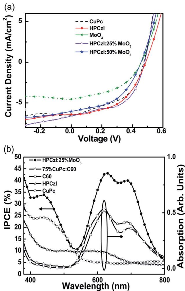
Fig. 2 (a)  $J$ - $V$  curves for devices with CuPc, HPCzI, MoO<sub>3</sub> and HPCzI:  $Y\%$  MoO<sub>3</sub> as anode buffers,  $Y = 25, 50$ . (b) The IPCE of device with structure of ITO/HPCzI: 25% MoO<sub>3</sub> (15 nm)/75% CuPc:C60 (25 nm)/C60 (20 nm)/TPBi (8 nm)/Al (100 nm), and the film absorptions of C60, HPCzI, CuPc and CuPc:C60 (3 : 1).
