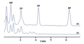
Fig. 8 HPLC chromatograms of four paraben compounds in real pond water sample after MSPE, blank (a) with spiked 100  $\mu$ g L<sup>-1</sup> (b). Extraction conditions were in optimal condition. Peak identification: methyl paraben (MP), ethyl paraben (EP), propyl paraben (PP), and butyl paraben (BP).
