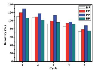
Fig. 9 Extraction recoveries of IL-MNP-BCD-TDI adsorbent in 5 different run.
