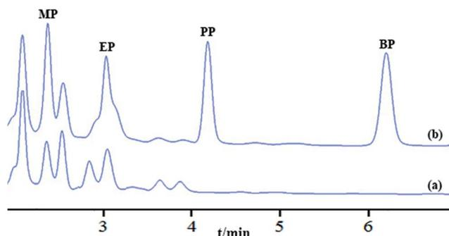
Fig. 8 HPLC chromatograms of four paraben compounds in real pond water sample after MSPE, blank (a) with spiked  $100 \mu\text{g L}^{-1}$  (b). Extraction conditions were in optimal condition. Peak identification: methyl paraben (MP), ethyl paraben (EP), propyl paraben (PP), and butyl paraben (BP).
