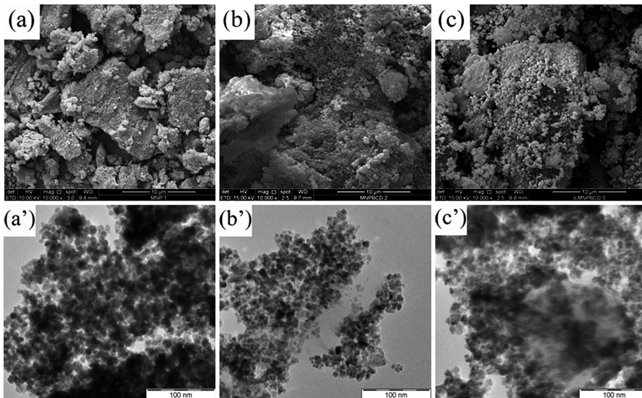
Fig. 4 SEM image of (a) MNP, (b) MNP- $\beta$ CD-TDI and (c) IL-MNP- $\beta$ CD-TDI, and TEM image of (a') MNP, (b') MNP- $\beta$ CD-TDI and (c') IL-MNP- $\beta$ CD-TDI.
