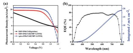
Fig. 5 (a) Current (J)-voltage (V) curves of the solar cells with SDF-OMeTAD and spiro-OMeTAD under AM 1.5 conditions (100 mW cm<sup>-2</sup>). (b) EQE spectra of CH<sub>3</sub>NH<sub>3</sub>PbI<sub>3</sub>/SDF-OMeTAD perovskite solar cell.
