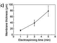
Fig. 3 Modulation of the properties of electrospun nanofiber membrane: nanofiber diameter variation (a) and pore size variation (b) with respect to the PCL concentration. (c) Membrane thickness variation with respect to the electrospinning time. Error bar presents the standard deviations of measured values.
