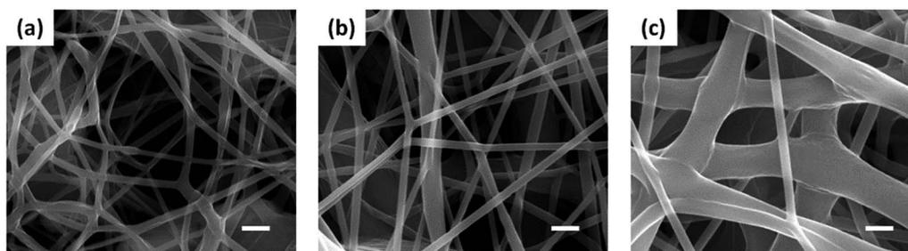
**Fig. 2** SEM images of electrospun PCL nanofiber membranes fabricated with PCL aqueous solutions with concentrations of 6 (a), 7 (b), and 8 wt% (c). Scale bar represents 1  $\mu\text{m}$ .
