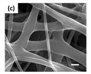
Fig. 2 SEM images of electrospun PCL nanofiber membranes fabricated with PCL aqueous solutions with concentrations of 6 (a), 7 (b), and 8 wt% (c). Scale bar represents 1  $\mu$ m.
