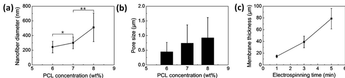
**Fig. 3** Modulation of the properties of electrospun nanofiber membrane: nanofiber diameter variation (a) and pore size variation (b) with respect to the PCL concentration. (c) Membrane thickness variation with respect to the electrospinning time. Error bar presents the standard deviations of measured values.
