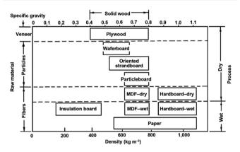
Fig. 1 Classification of wood-based panels.<sup>17</sup>
