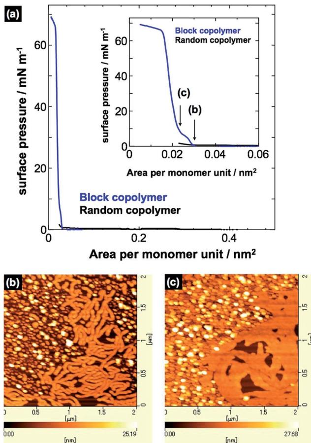
Fig. 4 (a)  $\pi$ -*A* isotherms of PVCa-*ran*-PSt and PVCa-*b*-PSt. AFM images of surface micelles of PVCa-*b*-PSt transferred onto mica substrates at (b) 1 mN m<sup>-1</sup> and (c) 10 mN m<sup>-1</sup>.
