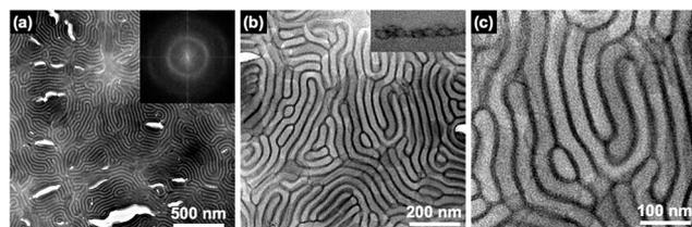
Fig. 3 TEM images of PVCa-*b*-PSt ultrathin films formed at the air–water interface at different magnifications (a) 8k, (b) 20k and (c) 40k, respectively. The PVCa domains were stained with OsO<sub>4</sub>. Inset images show an (a) FFT image and (b) cross-sectional TEM image of the ultrathin film.
