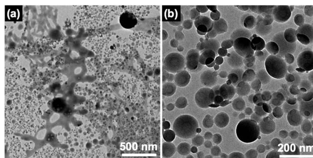
Fig. 2 TEM images of PVCa-*ran*-PSt network-like (a) and spherical (b) aggregates formed at the air–water interface. The PVCa domains were stained with OsO<sub>4</sub>.
