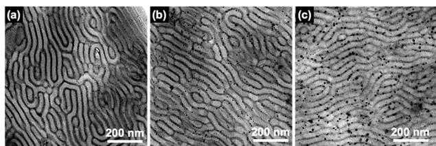
Fig. 7 TEM images of ultrathin films of PVCa-*b*-PSt immersed in aq. AgNO<sub>3</sub> for (a) 1 h, (b) 2 h, and (c) 4 days. The PVCa domains were stained with OsO<sub>4</sub>.
