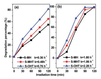
Fig. 5 Photocatalytic activities of the samples  $(0.1\,\mathrm{g})$  for (a) phenol and (b) 4-CP degradation under UV light irradiation.
