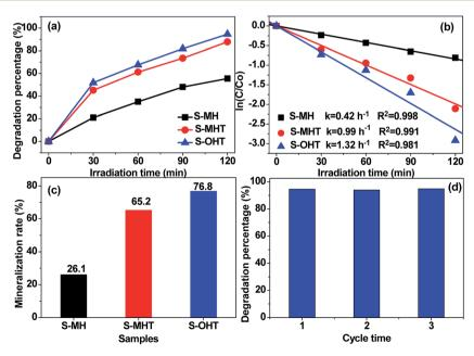
Fig. 4 (a) Photocatalytic degradation curves of BPA (20 mg  $L^{-1}$ ) for different samples (0.1 g) under UV light irradiation; (b) kinetic plots of  $L^{-1}$ 0 vs. irradiation time; (c) mineralization rate of BPA by different samples under UV light irradiation for 2 h; (d) cycling runs of S-OHT for BPA degradation under UV light irradiation.
