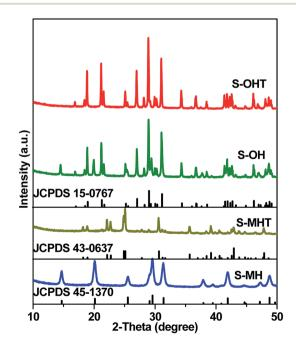
**Fig. 1** XRD patterns of the as-synthesized S-MH, S-MHT, S-OH, S-OHT, together with the standard patterns of h-BiPO<sub>4</sub> (JCPDS 45-1370), m-BiPO<sub>4</sub> (JCPDS 43-0637) and n-BiPO<sub>4</sub> (JCPDS 15-0767).
