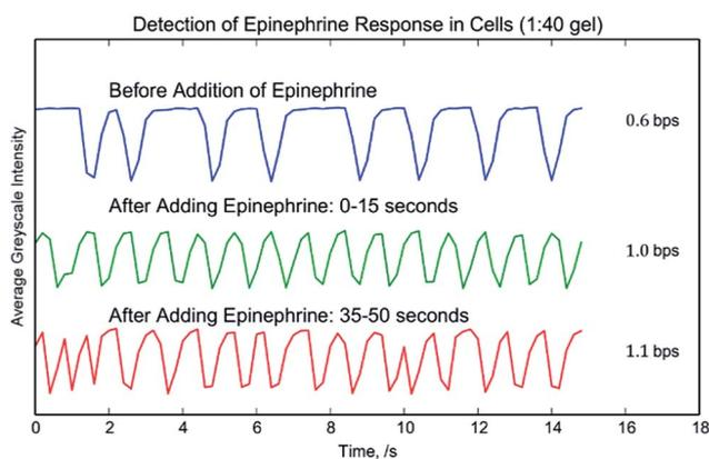
**Fig. 12** Cardiomyocyte and epinephrine beating rate. The beating of cardiomyocytes on a diffraction grating substrate was recorded by Video, S8.† The graph shows the average greyscale value of the video at different times during the experiment. After adding epinephrine the beating rate increases and the beating rate remains consistent over the course of the video. The crosslinking agent : base ratio for the substrate was 1 : 40.
