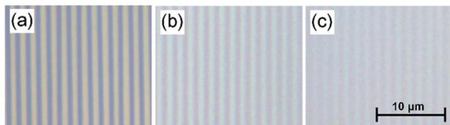
Fig. 4 Microscopic image of surface structure of CD and PDMS gratings. The diffraction pattern of the (a) CD and PDMS gratings are visible under the microscope. The mixing ratios of the PDMS gels are (b) 1 : 35, and (c) 1 : 50. The softer gel (1 : 50) produces a lower contrast pattern.
