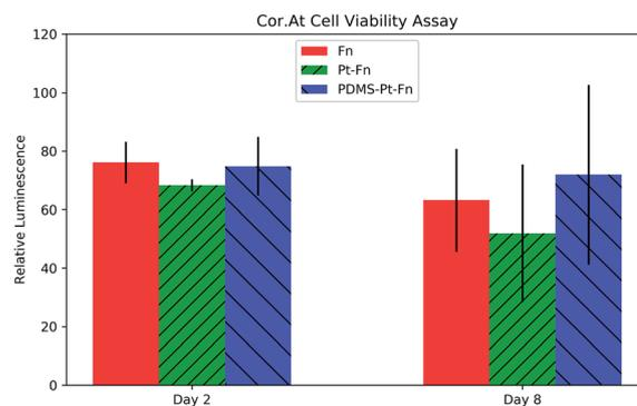
**Fig. 10** Cor.At Viability. Cor.At cells were seeded on 8-well plates coated with: platinum and fibronectin (Pt-Fn); PDMS, platinum and fibronectin (PDMS-Pt-Fn); and fibronectin as a control (Fn). After performing the CellTiter-Glo 2.0 assay the luminescence of the medium is proportional to cell quantity. No evidence of toxicity from PDMS or platinum is detected after eight days. Sample luminescence is normalized to an empty well without cells.
