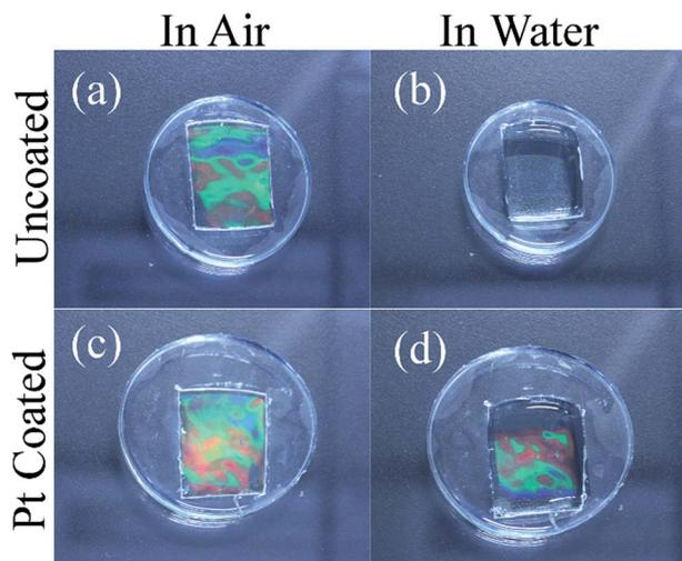
**Fig. 8** Diffraction grating gel and effect of platinum coating. PDMS grating when observed (a) in air and (b) in water. Platinum (Pt) coated PDMS grating when observed (c) in air and (d) in water. The Pt layer increases the visibility of the diffraction pattern and allows it to be observed even when submerged. Sylgard 184 PDMS diffraction gratings were prepared with a curing agent/base weight ratio of 1 : 35.
