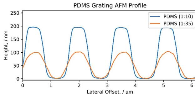
Fig. 6 AFM profile of PDMS grating. Cross-section profile of both a (1 : 10) and (1 : 35) PDMS diffraction grating.
