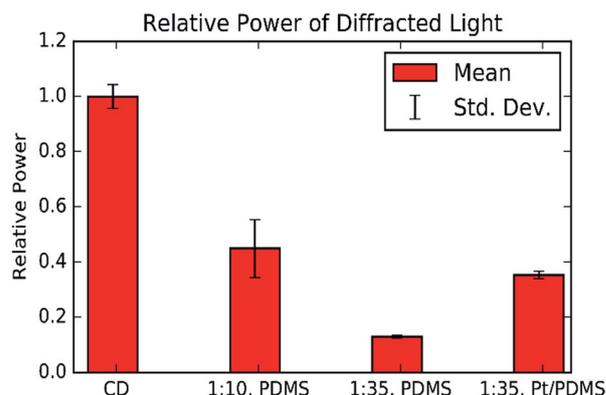
Fig. 7 Power of diffracted light from CD and PDMS samples. The power of the first order diffracted beams is compared between a CD piece, a (1 : 10) PDMS grating, a (1 : 35) PDMS grating, and a platinum (Pt) coated (1 : 35) PDMS grating. The softer PDMS produces lower power diffracted light, however, the Pt coating appears to restore much of the intensity lost due to the softness of the (1 : 35) PDMS.
