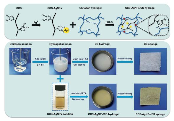
Fig. 1 Schematic representation and preparation procedure for CCS-AqNPs/CS sponges.
