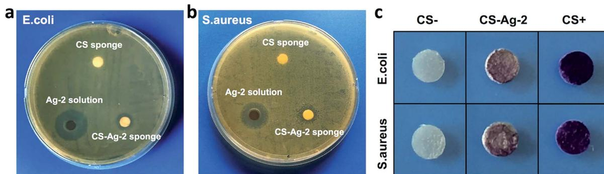
Fig. 5 Inhibition zones of CS sponge, CS-Ag-2 sponge and Ag-2 solution against *E. coli* (a) and *S. aureus* (b), Ag-2 is a CCS-AgNPs solution containing the same silver amount as CS-Ag-2 sponge; (c) photos of samples stained by crystal violet after disc diffusion test.
