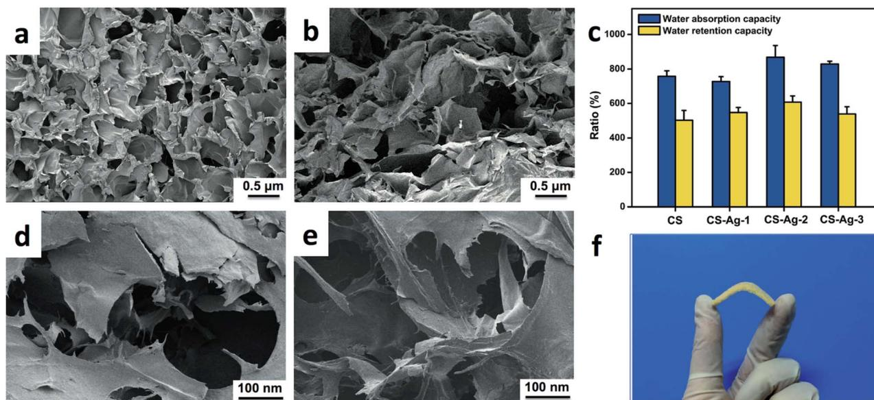
Fig. 3 SEM images of sponges: (a, d) CS sponge; (b, e) CS-Ag-2 sponge; (c) the water absorption and retention capabilities of CS, CS-Ag-1, CS-Ag-2, and CS-Ag-3; (f) photo shows the flexibility of CS-Ag-2 sponge.
