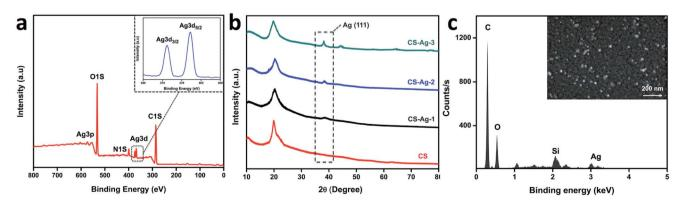
Fig. 2 (a) XPS fully scanned spectra of CS-Ag-2 and XPS spectra of Ag 3d; (b) XRD patterns of CS, CS-Ag-1, CS-Ag-2, and CS-Ag-3; (c) insert shows a SEM image of CS-Aq-2 sponge and EDS spectra corresponded to the SEM image
