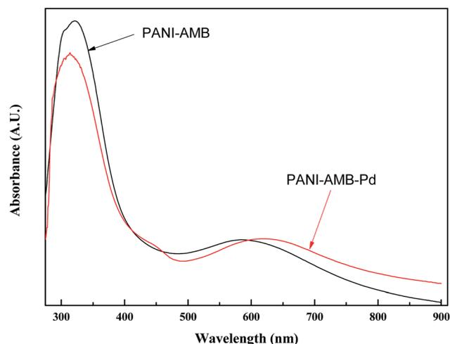
Fig. 13 UV-vis spectra of PANI-AMB, and PANI-AMB-Pd.
